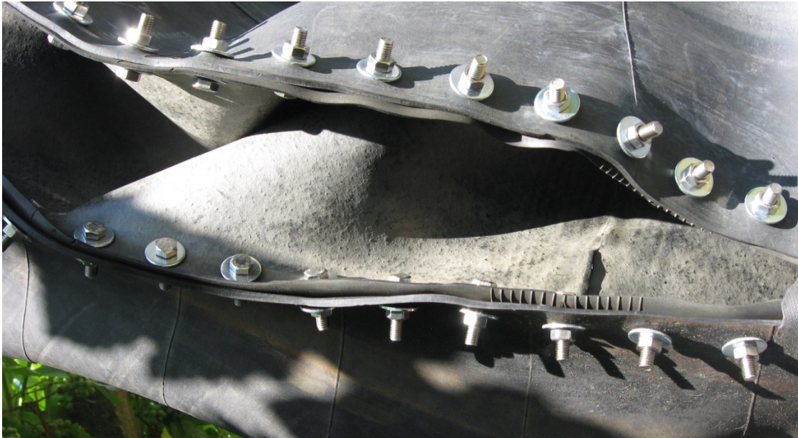
Figure 6 Inner tube detail showing powdery lining. 2008
