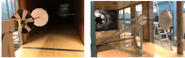
Fig. 5. The wind tunnel setup, with a paper origami model mounted on a free-spinning axle that spins with a code disk used for spin rate measurement.
