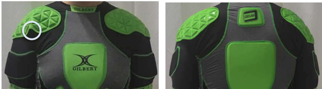
Figure 46: Front and back view of garment C fitted to participant 6; a region that lift away from the body is circled (Authors Own Image, 2018)
