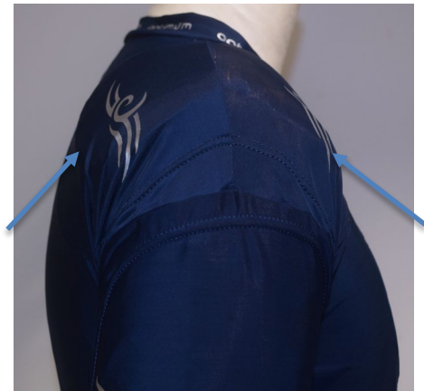
Figure 65: HC005 (non-auxetic comparison) inserted within the pocketed region of a rugby top and fitted to a size XL men's mannequin (Authors Own Image, 2019)
