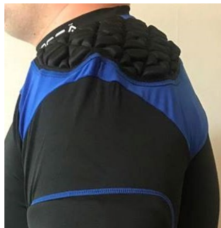
Figure 43: Lefthand side view of the vacuum moulded shoulder pads fitted to the participant (Authors Own Image, 2017)
