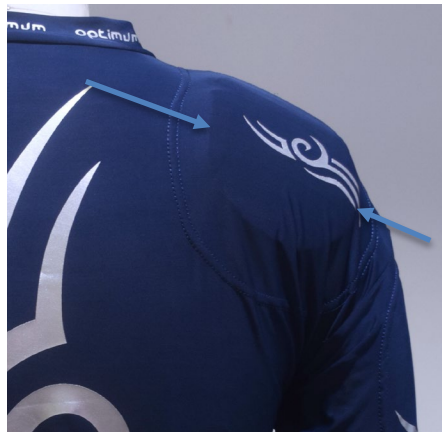
Figure 65: HC005 (non-auxetic comparison) inserted within the pocketed region of a rugby top and fitted to a size XL men's mannequin (Authors Own Image, 2019)
