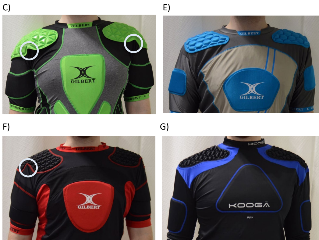
Figure 45: Front view of vacuum moulded shoulder pads fitted to participant 4; regions that lift away from the body are circled (Authors Own Image, 2018)
