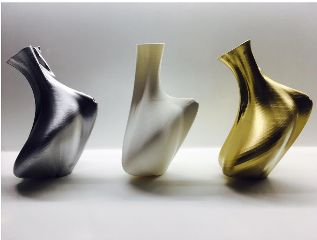
Figure 105 First stage neo ebreeq 3D printed prototypes, using PLA filament
