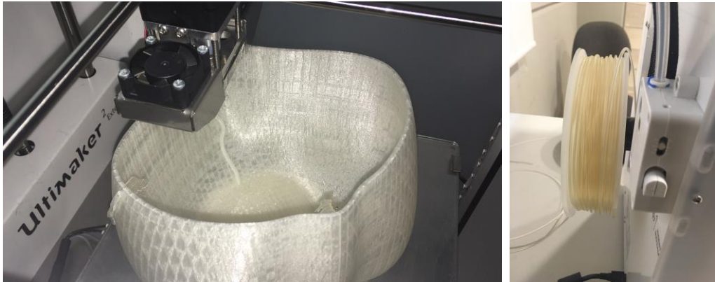
Figure 100 3D printing the neo ebreeq with layers of PLA material
