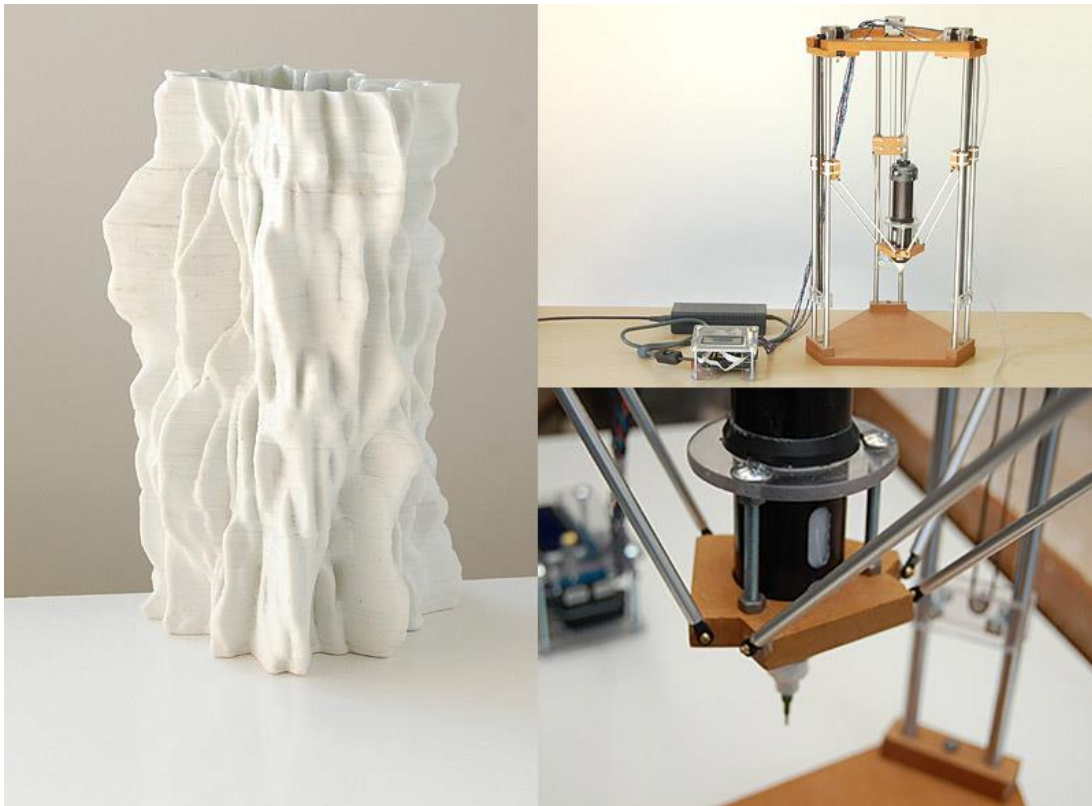
Figure 69 Sculpture by Jonathan Keep (left) using ceramic 3D printer (right) Image retrieved from Design-milk https://design-milk.com/artist-jonathan-keep-sculpts-pottery-using-ceramic-3d-printer/3d-ceramic_pottery_printer/
