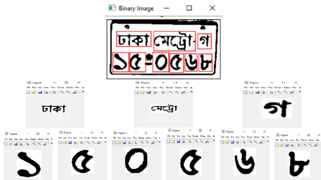
Figure 12. Example of character segmentation from a vehicle number plate.
