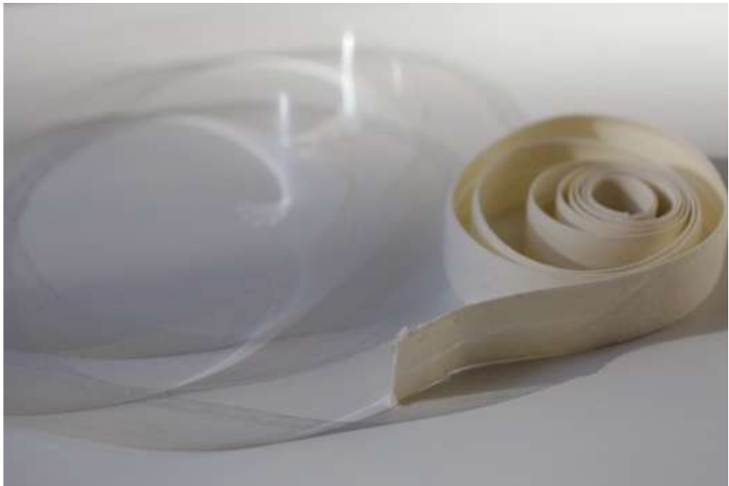
Figure 59. Clear film leader spliced to fabric ribbon. Mary Stark, 2013
