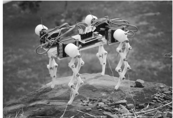
FIGURE 2. Felis - A Planar Reconfigurable Quadruped Robot.
