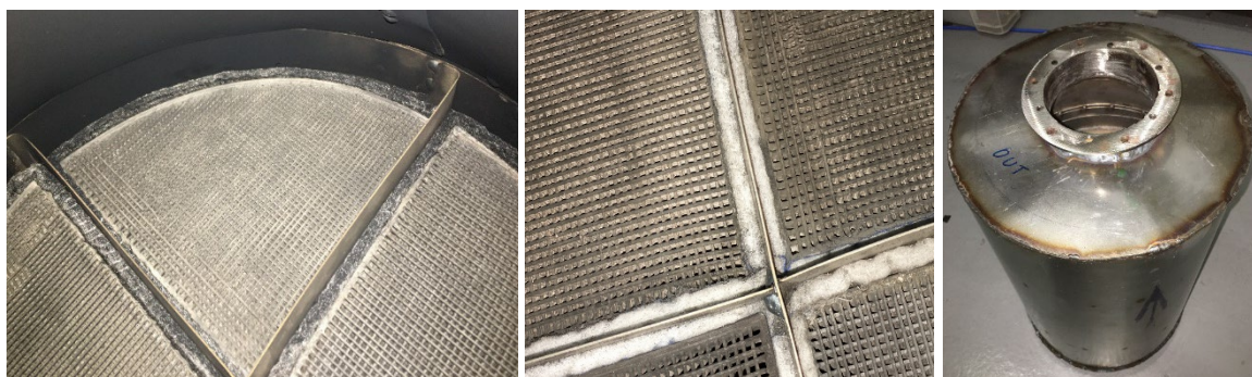
Figure 5. 3D printed substrate washcoated and canned for testing as DOC.
