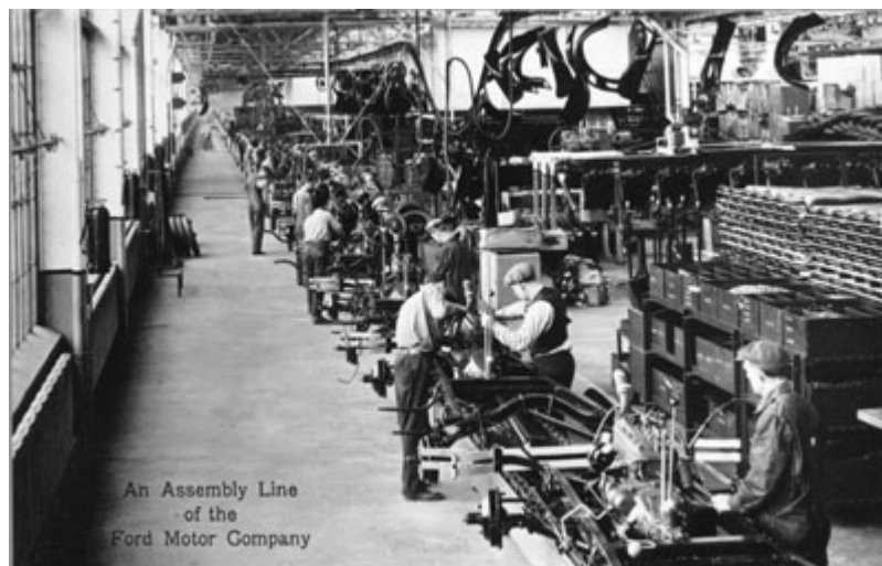
Figure 4. Flow line production of Model T. Source: Ford
