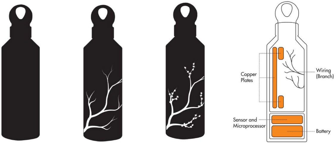
Figure 2: States of the bottle and technical details
