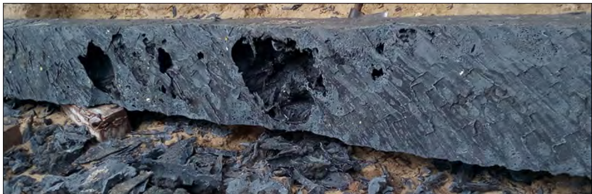
Figure 4. Poor quality plastic, holes the sizes of Mango's and Oranges!
