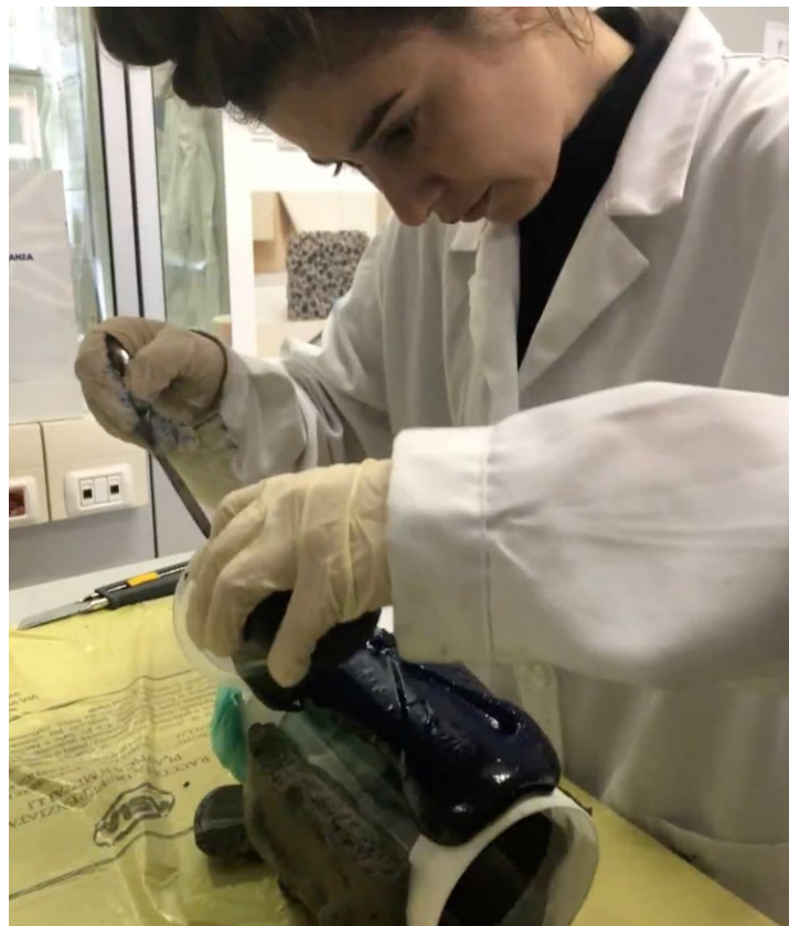
Figure 6. Designer pouring the foam with different techniques, speed and movements directly on cylindrical basic forms made of glass.
