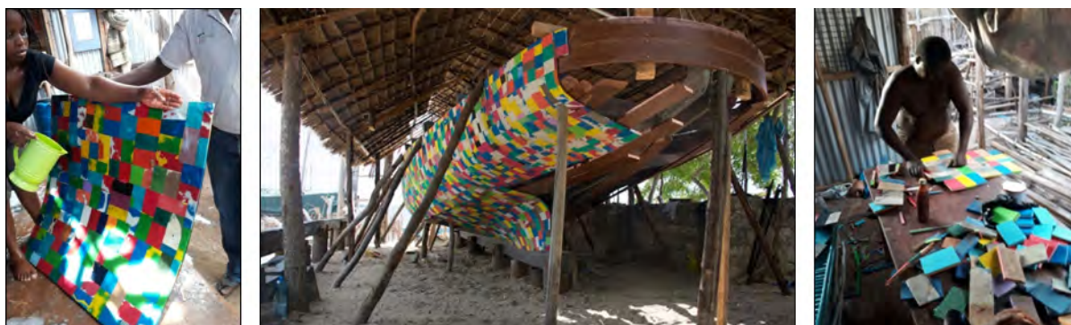
Figure 11. Images of the flipflop outer skin attached to the hull.
