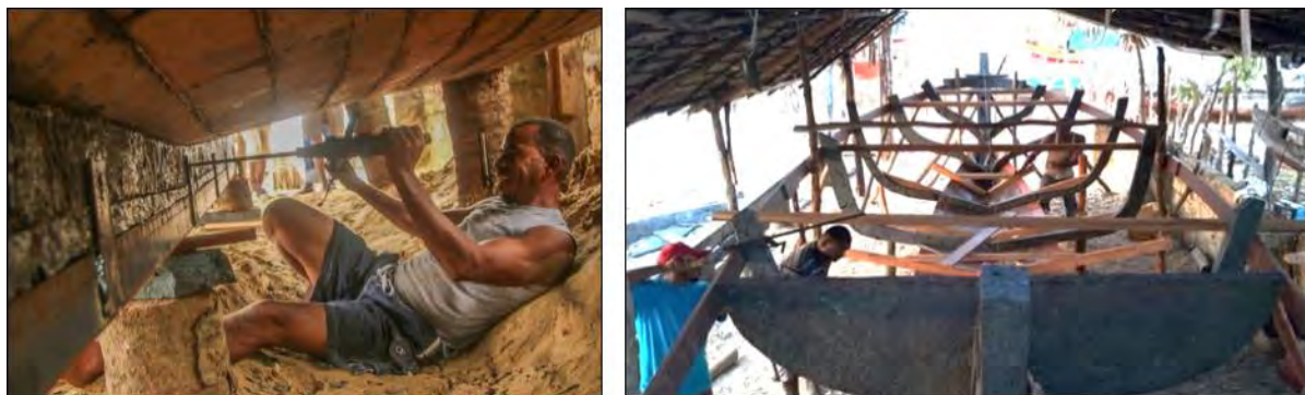
Figure 10. Images of the build process showing the internal structure.
