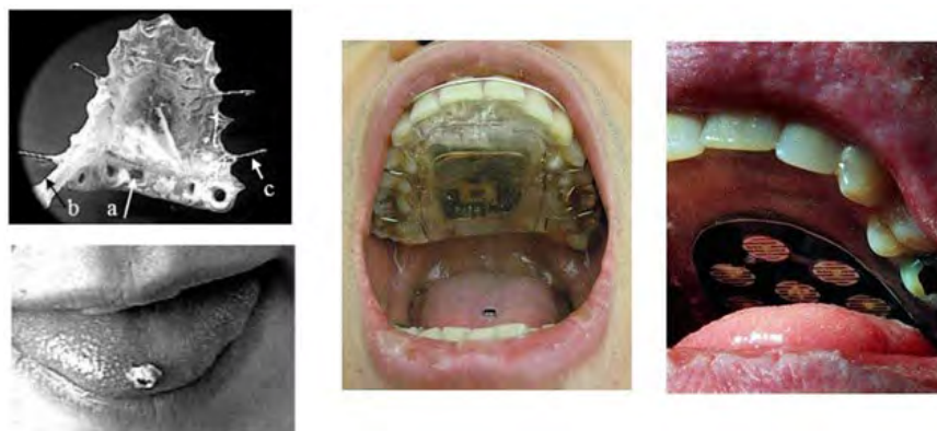
Figure.1 In-mouth control grants spinal cord injured users a way to interact with computer Source: assistivetech
