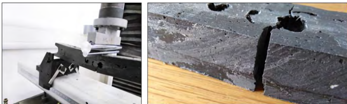
Figure 6. Cracks permeating through the sample material.
