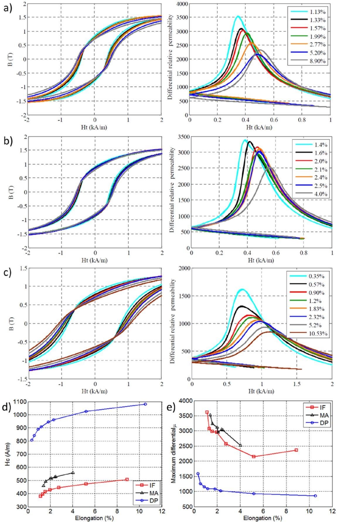
**Fig. 2.** BH loops and differential permeability curves for IF (a), MA (b) and DP (c) sample sets. Changes in coercive field (d) and maximum differential relative permeability (e) for increasing elongation
