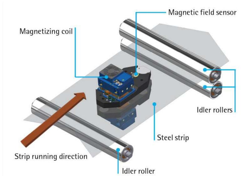
**Fig. 8.** Schematic diagram of IMPOC operating principle [5]
