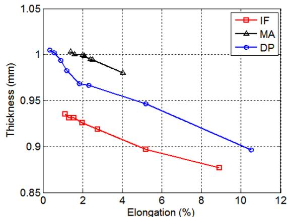
Fig. 1. Thickness for total percentage elongation for all sample sets
