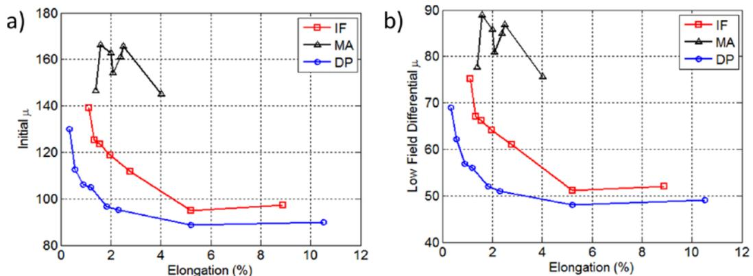
**Fig. 4.** a) Initial permeability derived from direct measurement of minor loops using U-core measurement system ( $\mu_i = \Delta B / \Delta H \cdot \mu_0$ ), b) Low field differential permeability derived from solenoid sensor
