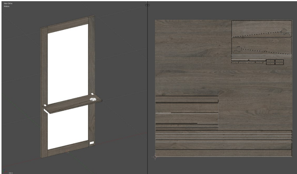
FIGURE 19 - A UV MAP AFTER HAVING THE CORRECT DIRECTION, SCALE AND LOCATION ON THE LAMINATE APPLIED
