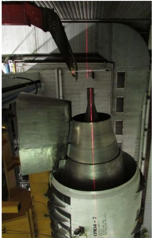
The engine was fueled with regular Jet A-1 (18.1% arom. and 13.6% H) and with a 32% HEFA blend (11.3% arom. and 14.1% H)
