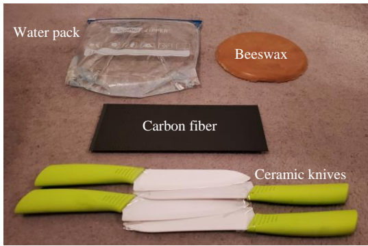
FIGURE 12. The materials that have been measured using the 20 GHz radiometer of Figure 11. From the top: the water pack (left), the yellow beeswax (right), the carbon fiber, and the ceramic. In the case of the ceramic, a larger surface area was created by fixing four (20 cm long bladed) ceramic knives together.
