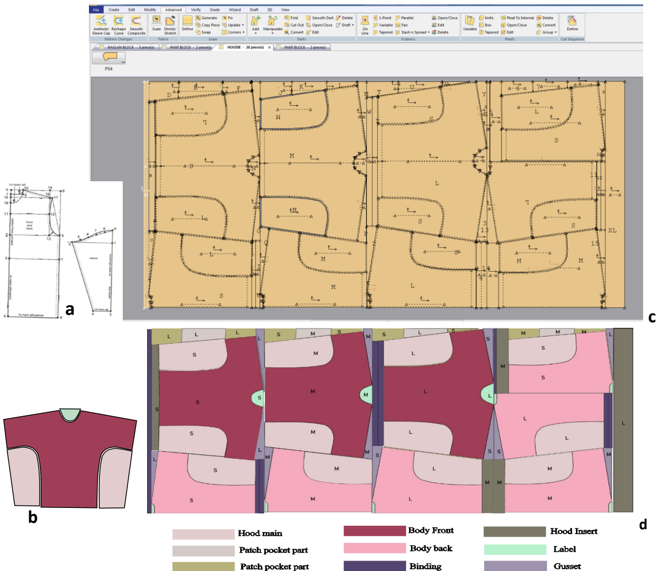
Figure 5: a) Silhouette of traditional patterns for t-shirt (Aldrich, 2011), b) silhouette of the chosen design, c) marker planning in the PDS widow, d) Coloured illustrations of all pattern pieces.
