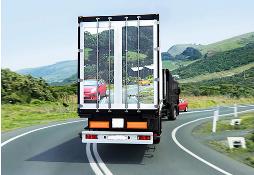
Fig. 7. See-through vision for a vehicle following a truck [111]
