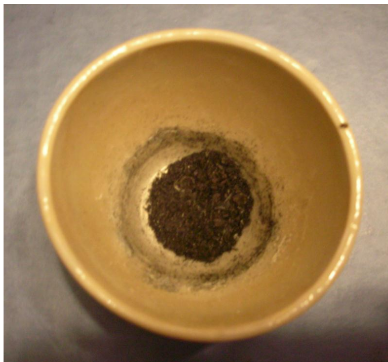
Fig 2.17: Photograph of SBA-15 top layer after CVD
