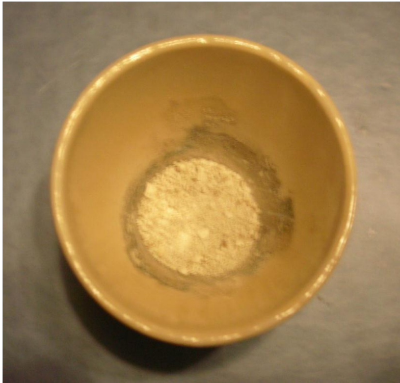
Fig 2.16: Photograph of SBA-15 prior to CVD
