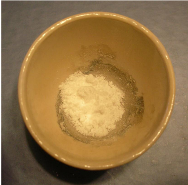
Fig 2.18: Photograph of SBA-15 lower layer after CVD
