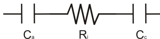
Figure 3.7 Basic circuit operations of a double layer capacitor.
