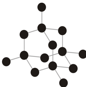
Figure 4.7 Schematic of sp^3 hybridised (tetrahedral) 'diamond' structure.
