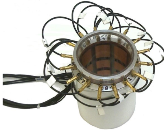
Figure 5.3 The 8 Electrode Sensor Array with Fitted Outer Shield
