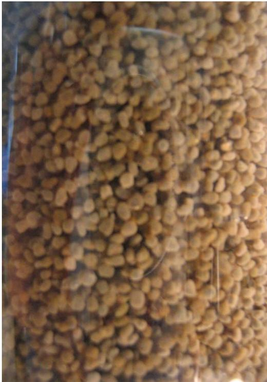
Fig. 2.3 Expanded bed column showing bioparticles in the expanded state, fully separated one from another in the upflowing wastewater.
