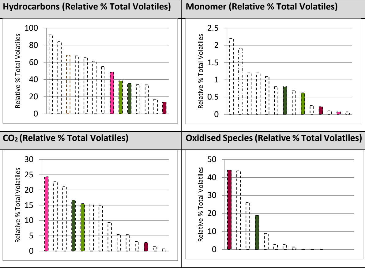
Figure 3.32: Volatiles as relative % total volatiles for polypropylene stabilised with formulations H, I, J and K, in air at 150°C for 2 hours by dynamic SPME-GC-MS
