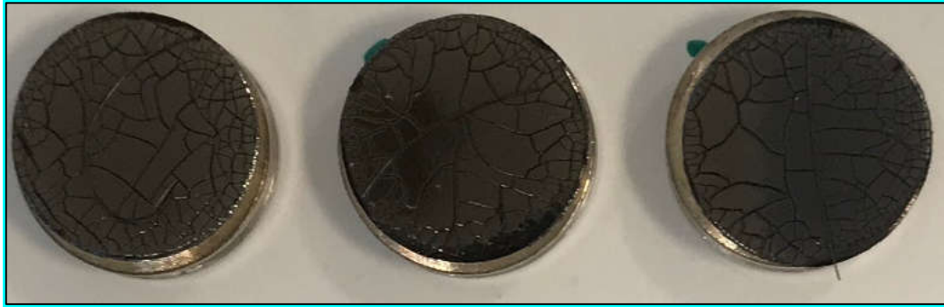
Fig.3.7 :The sputter coated samples of three different (Asian, African and European) hair strand samples.
