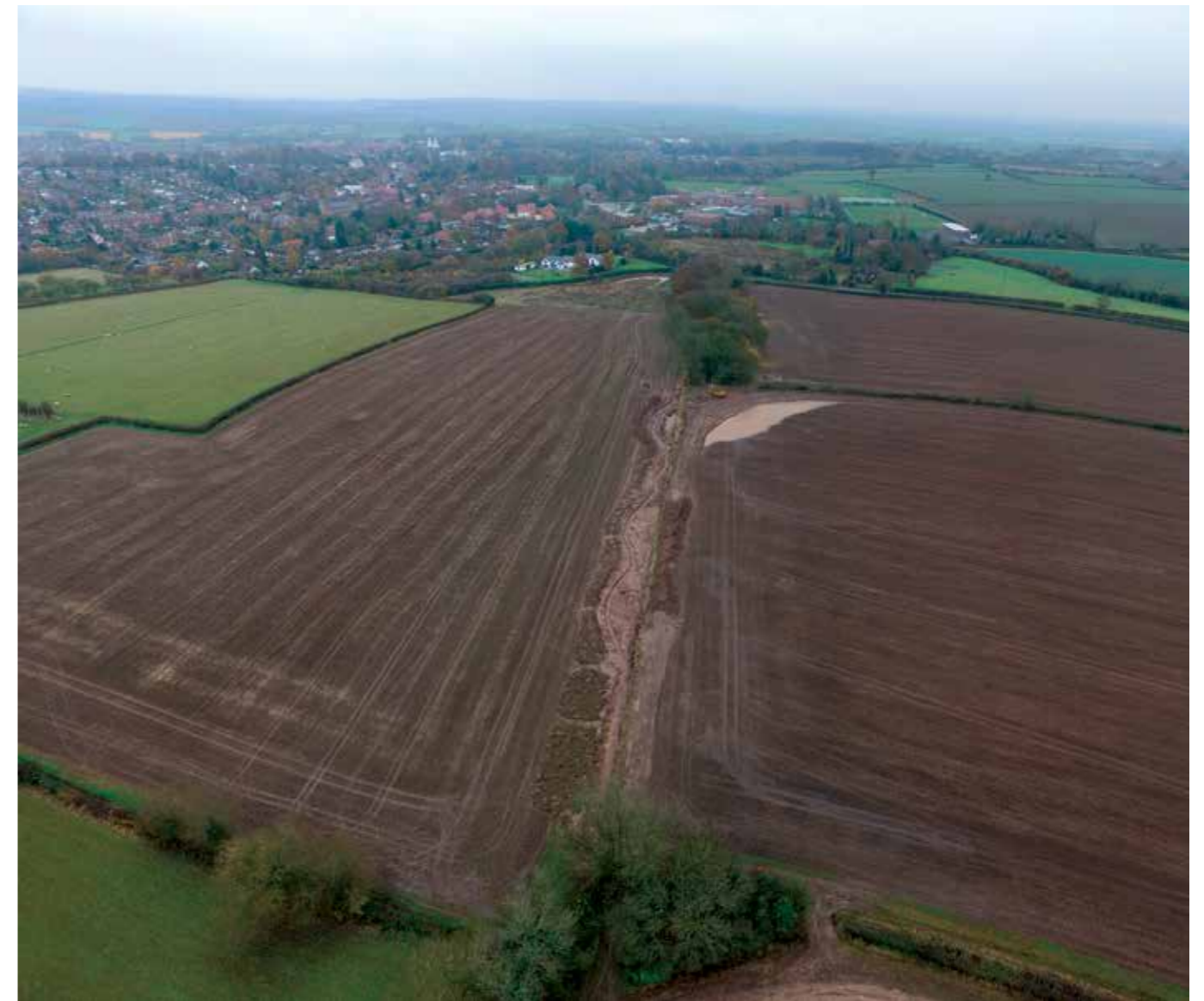
▲ Figure 2 Aerial image of the newly restored Springfield Dumble stream channel, and a constructed earth bund storing field surface water runoff following Storm Angus in November 2016 (© Dr Steven Godby).
