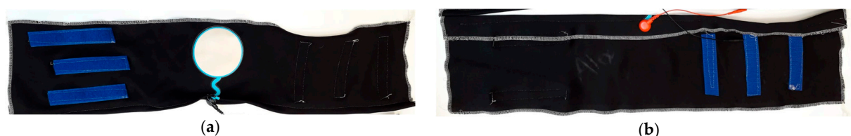
Figure 1. Images of the FES sleeve: (a) Front side with electrode and Velcro fastening; (b) Back side.
