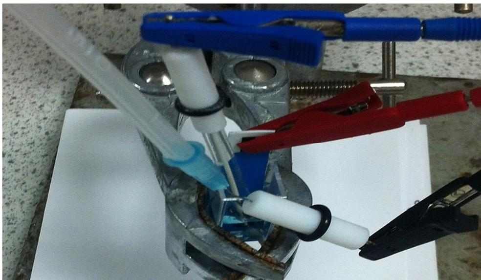
*Figure 4.1. Cuvette based three-electrode cell using a standard reference and counter electrode with an SPCE and facilitating the analysis of 1000 $\mu$ l volumes representative of the biosensor platform analytical cell.*
