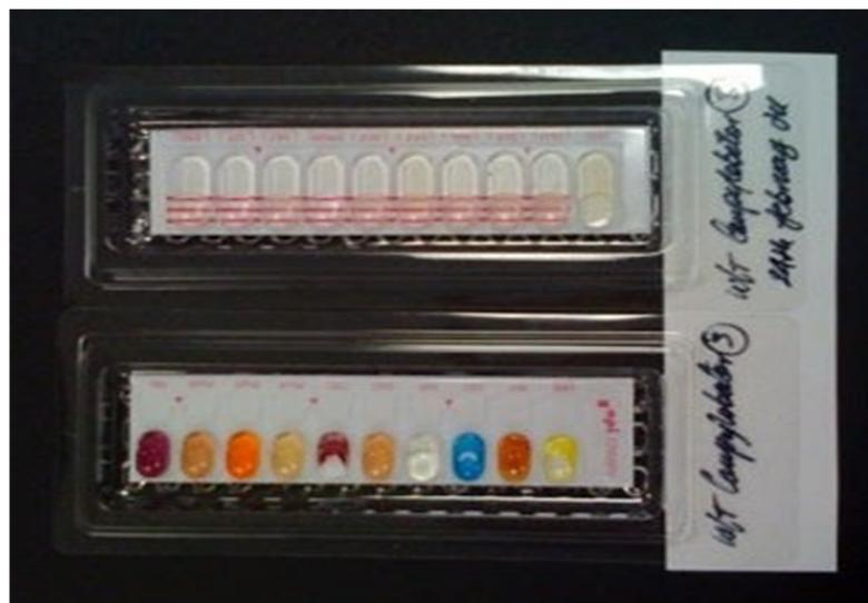
Figure 3.3. Typical API® strip, using colorimetric and binary test results to identify microbial species based on largely on their metabolic capacity. The colour indicator system makes API® strips ideal for high throughput automatic analysis.
