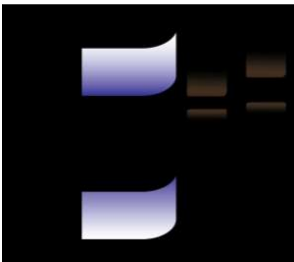
Figure 2. Band energy level diagram depicting the relevant energy levels of bulk PbSe and 6.5 nm PbSe QDs and the ZnO crystal. The energy positions for PbSe were calculated from reference 27.
