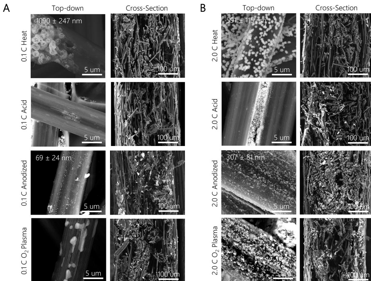
**Figure 4.** Top-down and cross-sectional backscattered-electron SEM micrographs of as-synthesized CoP electrodes at (A) low loadings (0.1 C of charge passed) and (B) high loadings (2.0 C of charge passed). The brighter regions represent the stronger electron scattering from higher Z number atoms (Co) in relation to the carbon support.
