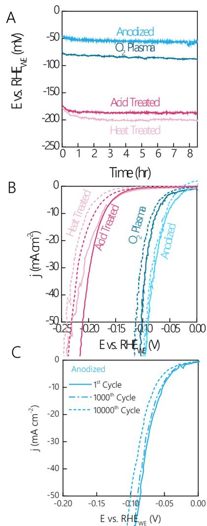
**Figure 2:** (A) Chronopotentiometric (CP) curves recorded at a constant current density of  $-10 \text{ mA cm}^{-2}$  for all low loading ( $0.1 \text{ C}$  of charge passed) CoP cathodes and (B) their respective cyclic voltammogram measurements before and after stability testing. (C) Accelerated durability testing for a CoP catalyst (low loading, anodized) at the 1<sup>st</sup>, 1000<sup>th</sup>, and 10000<sup>th</sup> cycle.
