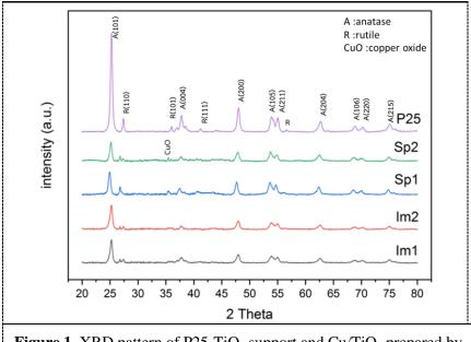
**Figure 1.** XRD pattern of P25-TiO<sub>2</sub> support and Cu/TiO<sub>2</sub> prepared by magnetron sputtering and conventional impregnation methods.
