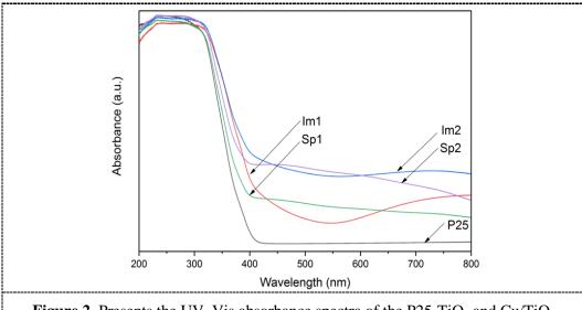
**Figure 2.** Presents the UV–Vis absorbance spectra of the P25-TiO<sub>2</sub> and Cu/TiO<sub>2</sub> prepared by using the magnetron sputtering and conventional impregnation methods.
