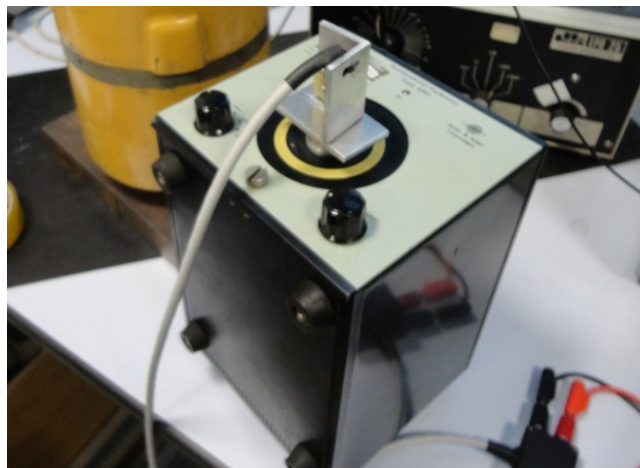
Figure 6-1 Accelerometer Calibrator with mounted ADXL001-70
