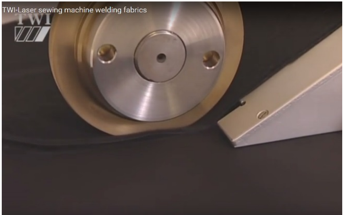
Laser welding a seam
