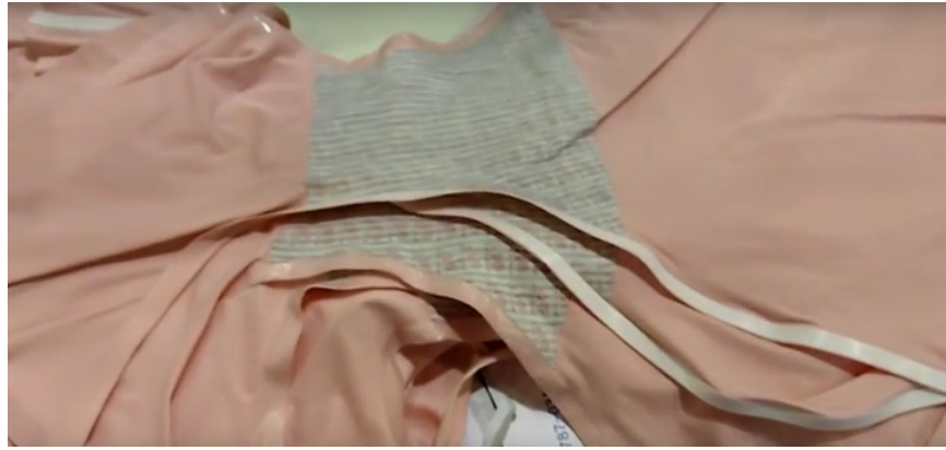
Lay down bonding strips on hem edges of briefs,
