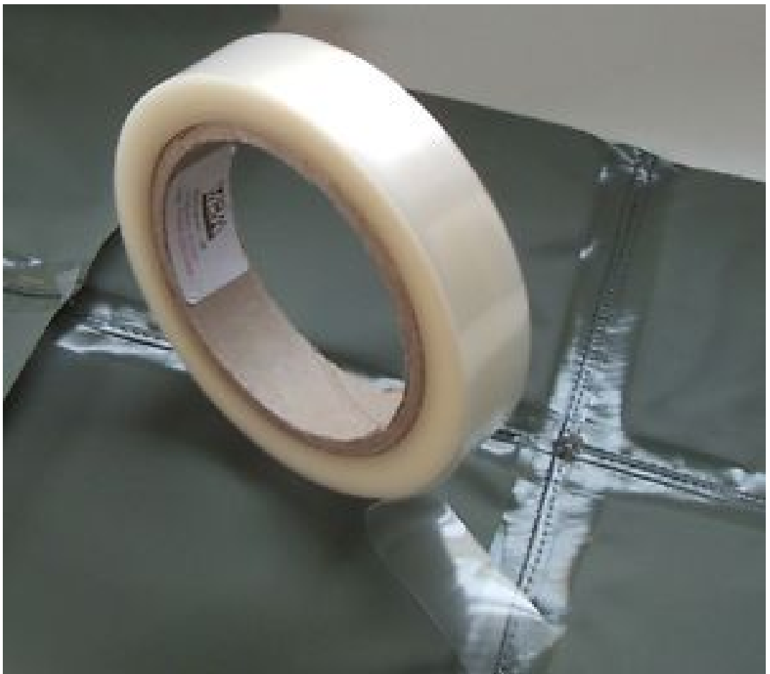
Sewn seams sealed with waterproof tape
