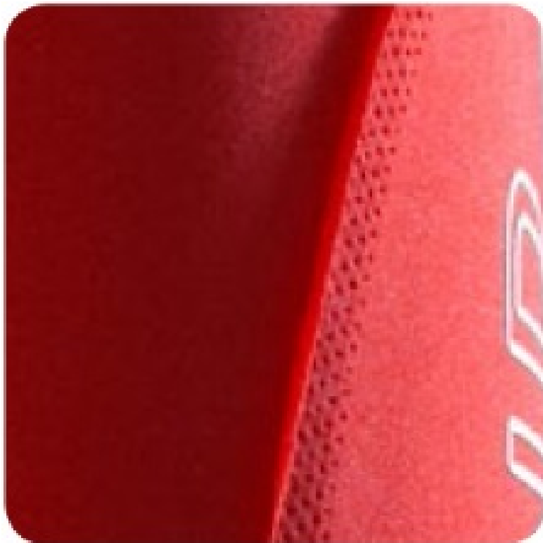
Ultrasonic cut & seal seam, http://www.pfaff-industrial.com Löffler ultrasonic welded seam,
