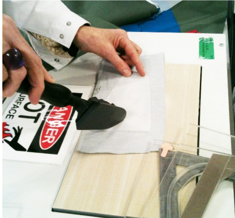
Pre-tacking preparation of bonding surfaces, E.Etheridge, 2013
