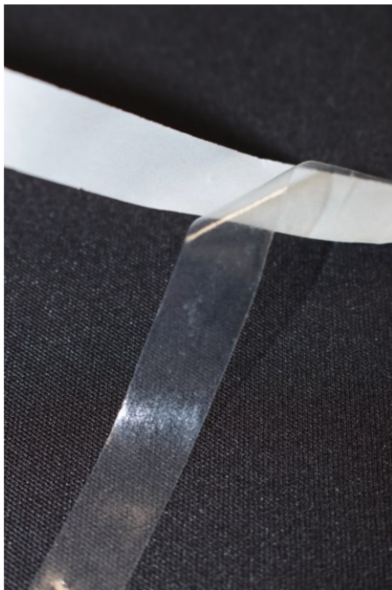
Bonding adhesive tape with release paper, E. Etheridge 2016
