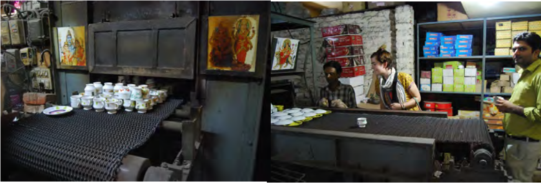
Images 52, 53: firing at Laxmi through the tunnel kiln
