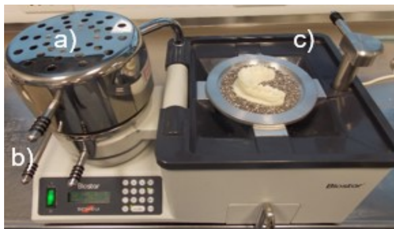
Figure 3-1: Thermoforming process of mouthguards; (a) heating chamber; (b) secured EVA blank; (c) participant's dental cast.
