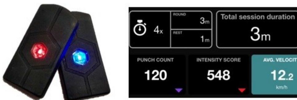
Figure 5-5: Left image shows two punch tracker sensors (Hykso®, Costa Mesa, California, US). Right image shows an example of the results for punch count, intensity score and average velocity following a 3-minute boxing round.
