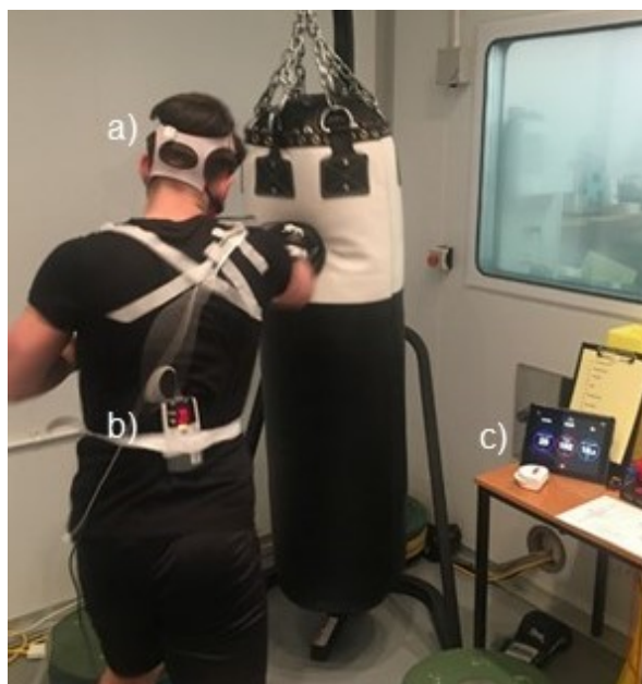
Figure 5-4: Participant performing a boxing-specific exercise protocol under hypoxic conditions; (a) mask connected to a breath-by-breath analyser; (b) pulse oximeter with wire connected to the ear lobe; (c) live feedback from punch tracker.
