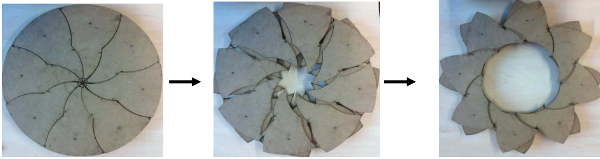
Figure 5.18: Prototyping two-dimension deployable structure constructed in Oita stadium (By author)
