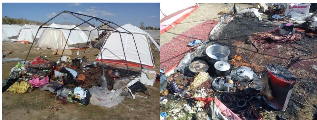
Figure 6.11: Burnt emergency shelter because of using unsafe material options for emergency sheltering. (Ref:www.varzeghanaras.blogfa.com)
