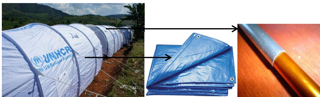
Figure 1.22: Tarpaulin as an existing water resistant material for coverage and Aluminium pole for structure
