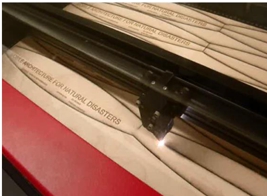
Figure 6.8: Screenshot of a video during prototyping strut deployable structure as an emergency shelter with board in laser workshop (By author).
