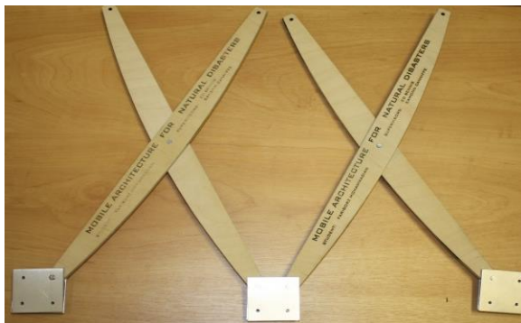
Figure 5.5: Experimenting deployable structure in scissor action in workshop (By author). Figure 5.6: Rotation and erection of deployable structure with scissor action mechanism (By author).
