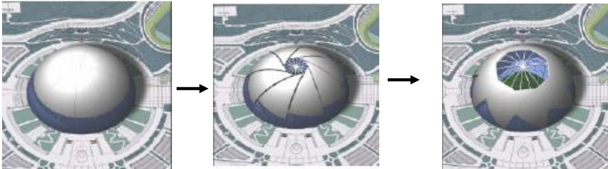
Figure 5.19: Three dimension deployable structure constructed as roof in Oita stadium (De Temmerman, 2007)
