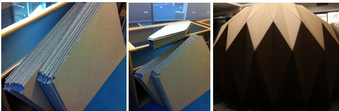
Figure 6.17: Thirty-two kilogram prototypes that was made by 120 cardboard panels (By author)
