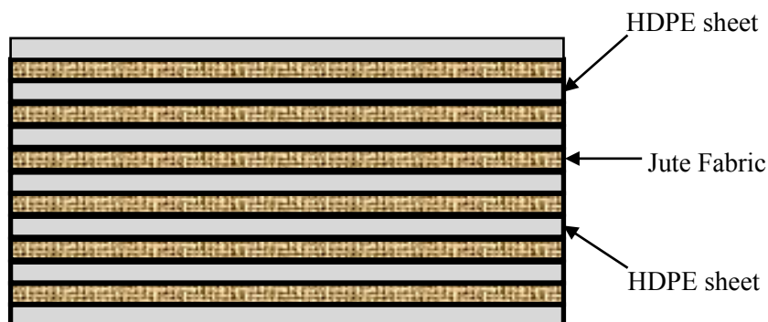
Fig. 1. 6-layer Jute-HDPE composite design
