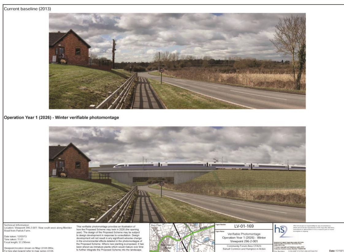
Figure 47. Example Phase 1 photomontage from the Environmental Statement for CFA 23, showing proposed embankment. The EIA for Phase 2b will have many such illustrations. This embankment, in a flood plain, was redesigned as a viaduct following input from local people.
