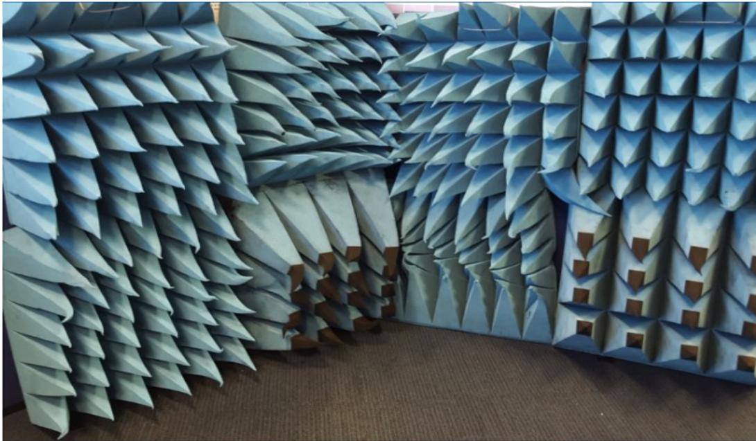
Figure 5.4: A wall of carbon loaded absorbing foam (length 1200 mm x width 2400 mm) surrounded the instrumentation.
