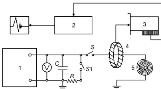
Fig.3 Diagram of pulsed *EMF* treatment circuit: 1 – high voltage supplier, 2 – processing software, 3 – analogue to digital convertor, 4 – coil, 5 – inductor, C – capacitor, R – ballast resistor, S – switches.
