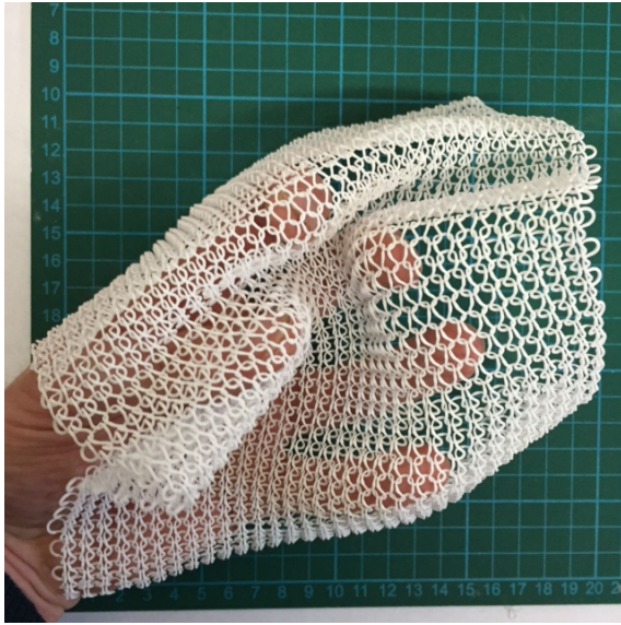
Figure 6. Flexibility of weft knitted piece.
