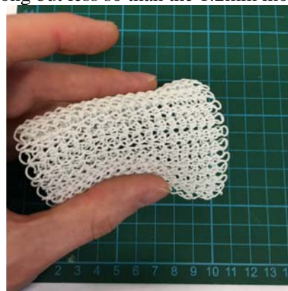
Figure 15. Flexibility of the interlock structure.
