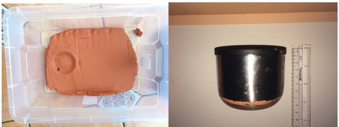
Figure 4.2 - a) (Left) Indent size in clay base and container. b) (Right) thermos lid used to make indent with size and clay markings.
