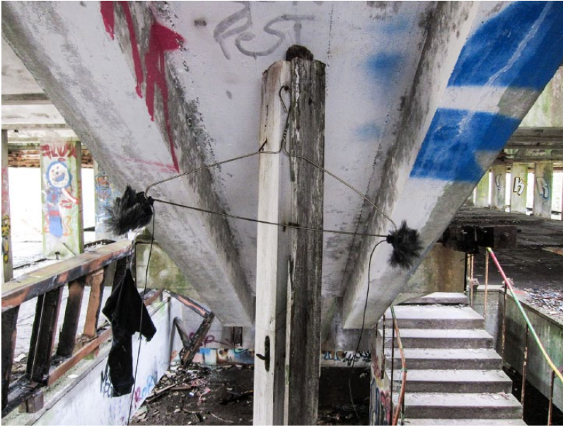
Figure 3. A spaced pair of miniature DPA 4060 omnidirectional microphones mounted on a wire coathanger and used to record an impulse response from the chapel area. The furry covers are Rycote wind jammers, used to prevent wind noise.
