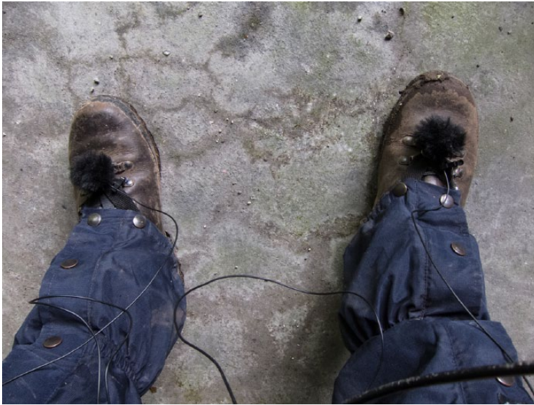
Figure 5. DPA 4060 microphones attached to walking boots to record footsteps and textures underfoot.
