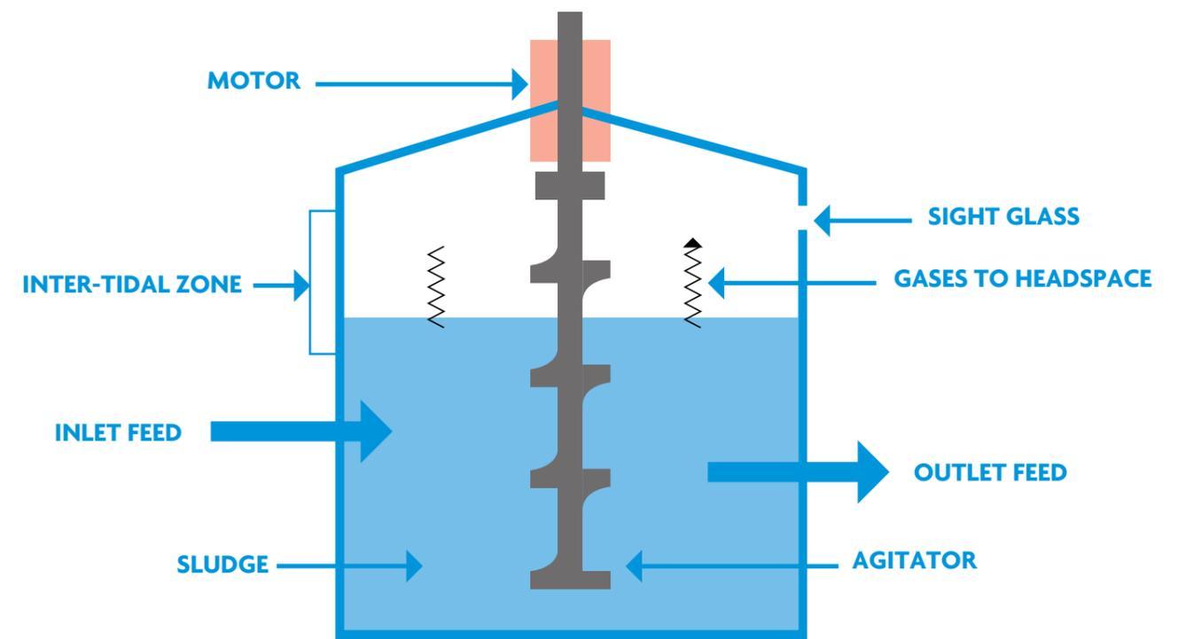
▲ Figure 1. Not-to-scale diagram of the hydrolysis tank.
