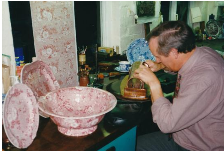
Fig. 3.81. Ken Collins engraving a ‘Primula’ pattern roller to create a ‘sheet’ pattern: a design with no distinct border. CHC.
