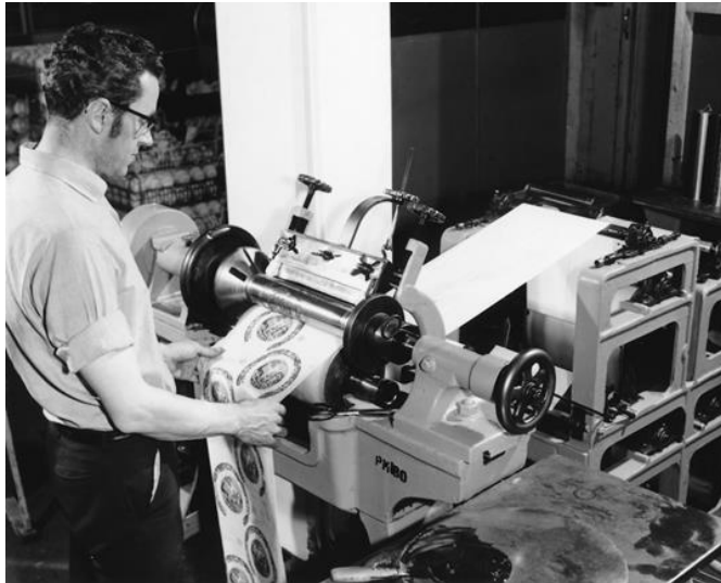
Fig. 3.80. Roller printing in action creating a continuous sheet of “Italian” pattern plates. CHC.
