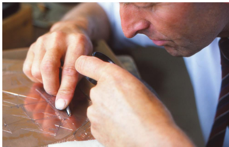
Fig. 3.19. Trevor Durose cutting an area of line-work: note the position of hands, graver, loupe and eye. CHC.
