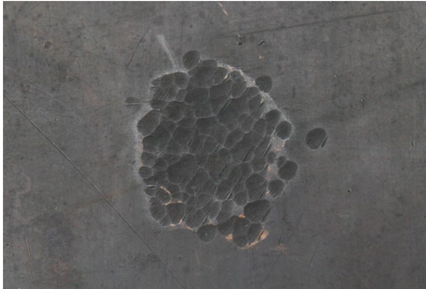
Fig. 3.29. Knocked-up area, showing hammer marks as tightly-grouped indentations.
