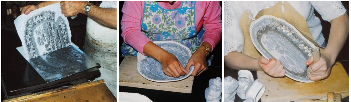
Fig. 1.11. The printed tissue is removed from the plate. 1.12. The pattern is cut out of the tissue and applied to the blank biscuit ceramic while the colour is wet. Fig. 1.13. The tissue pull is rubbed onto the ceramic with a stiff brush.
