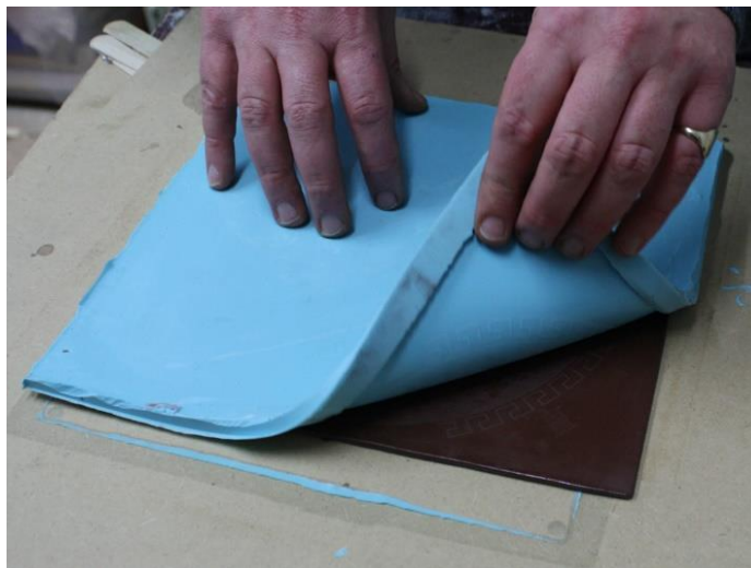
Fig. 6.110. The silicon mould is removed from the cured resin.
