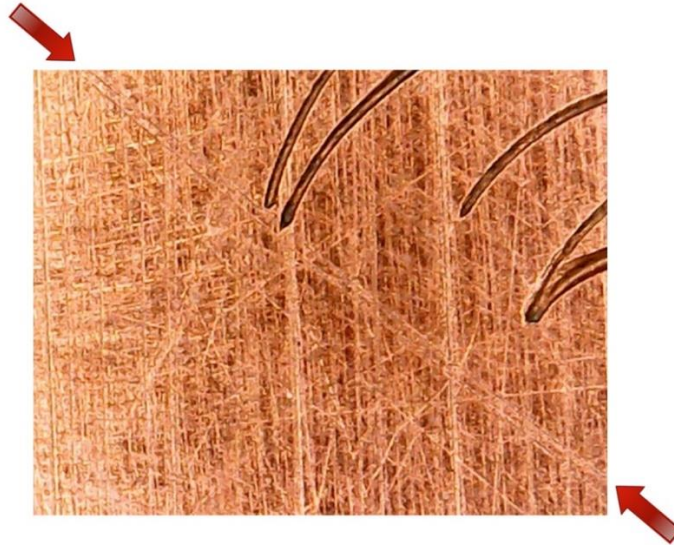
Fig. 6.140. Layout lines on a copper-plate.
