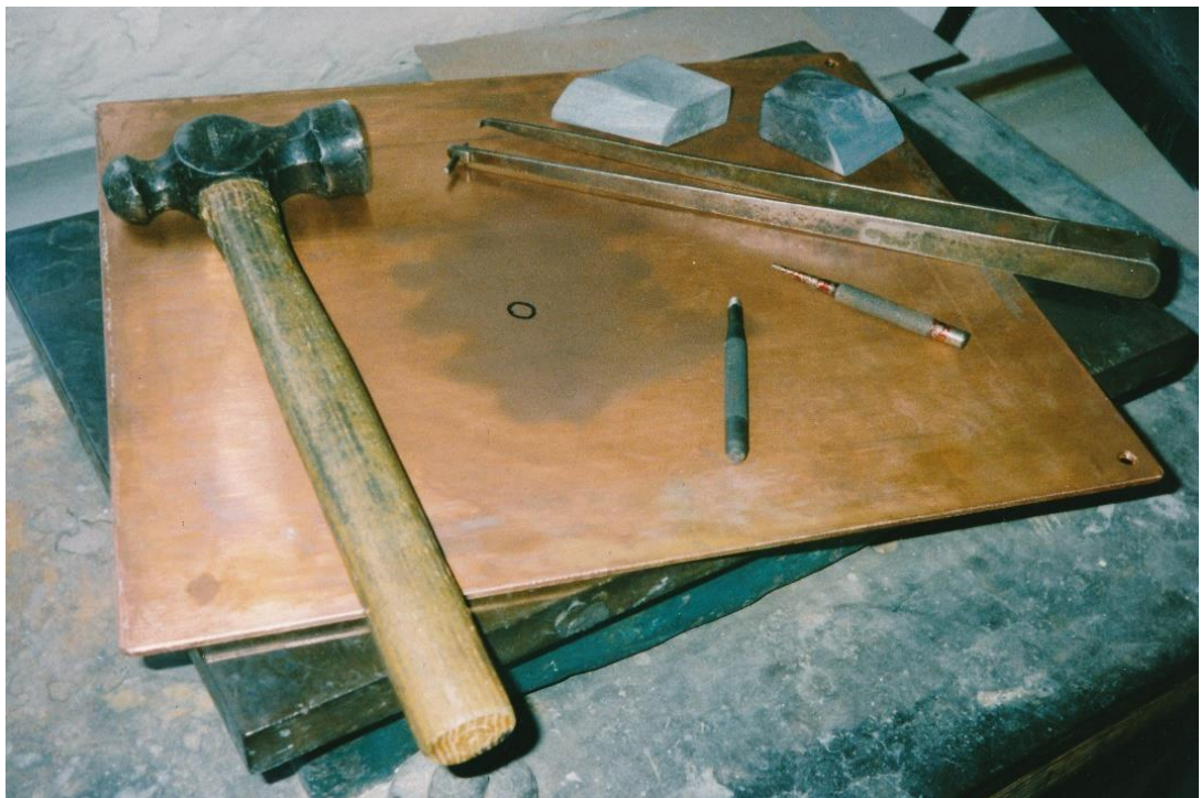
Fig. 3.28. Tools used for knocking-up and planishing, c.1980. CHC.
