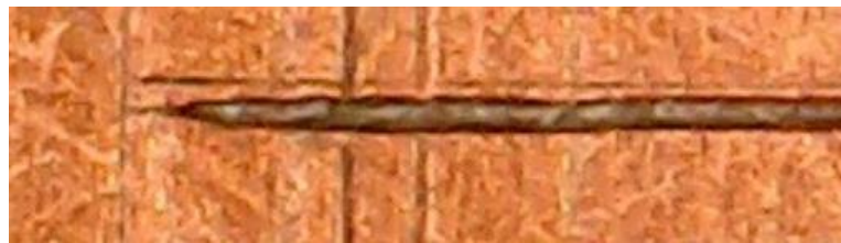
Fig. 6.151. Microscopy of a graver-cut line indicating manipulation by engraver.
