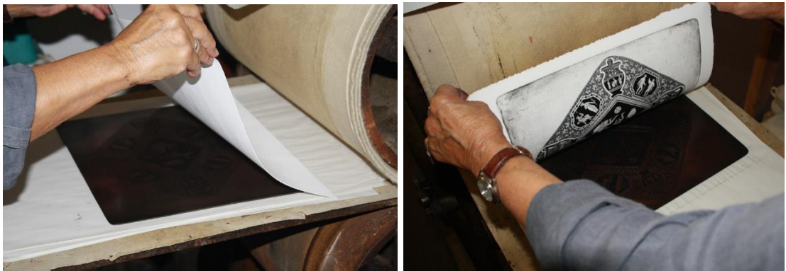
Fig. 6.67. Applying the paper, and Fig. 6.68, removing the paper after printing, 2015.
