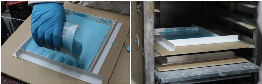
Fig. 6.100. The copper-plate is fully coated, and Fig. 6.101 placed in the oven to cure.
