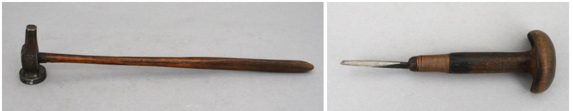
Fig. 3.113. A punching hammer, and Fig. 3.114. A graver.
