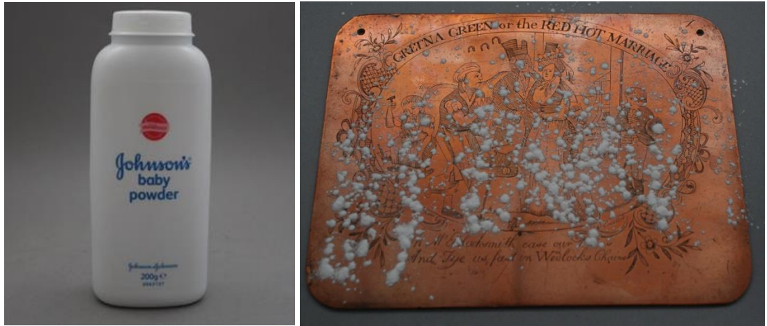
Fig. 6.10 and Fig. 6.11. Talcum powder and application to copper-plate.
