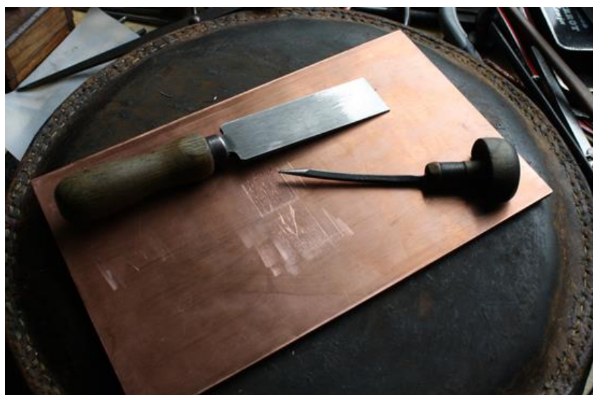
Fig. 2.45. A graver and scraper on my apprentice plate, 2015.
