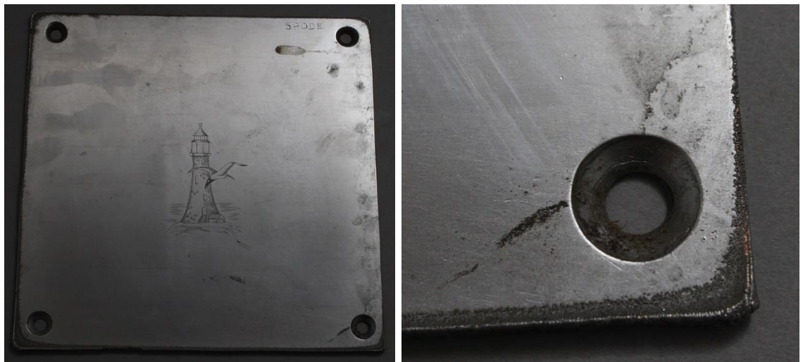
Fig. 3.5. and Fig. 3.6. Murray Curvex copper-plate, c.1970-90 and close-up of drilled holes.
