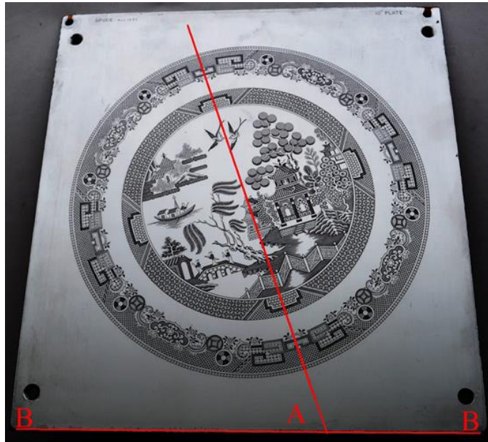
Fig. 3.105: An illustration of engraving orientation, c.1992. (CHC).
