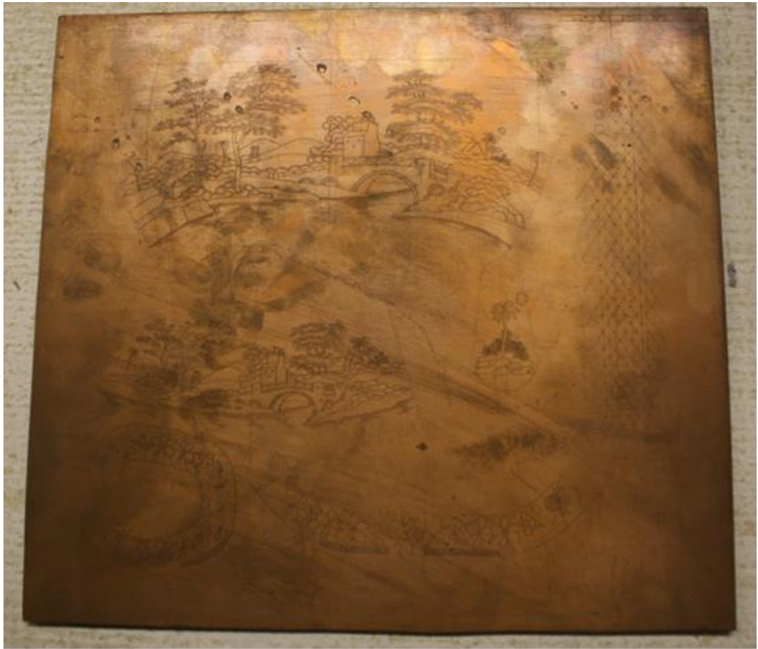
Fig. 3.87. Lay-out copper-plate used to create a “Tower” pattern coffeepot roller.
