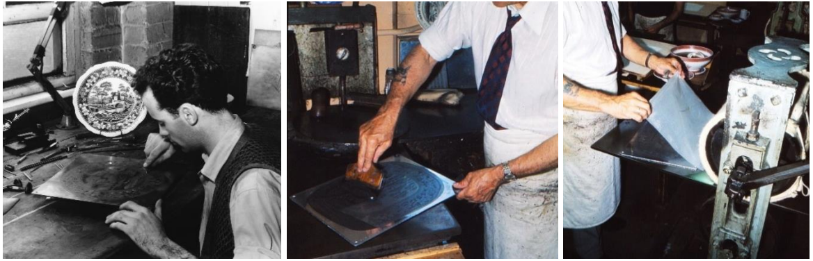
Fig. 1.8. A design being engraved onto a copper-plate. Fig 1.9. Cobalt-oxide printing colour is applied to the copper-plate. Fig. 1.10 The printing tissue, wet with printing size, is laid on to the colour-charged copper-plate and run through the printing press.
