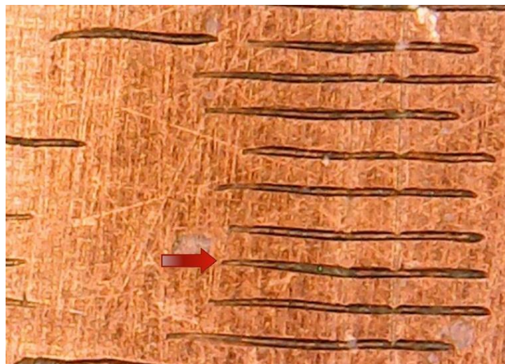
Fig. 6.141. Direction of line-work in an engraving.
