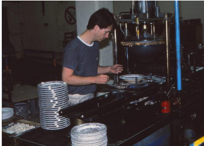
Fig. 3.99 (CHC). Printer, Rod Latham, using a gelatine pad (bomb) in the Murray Curvex machine to print 7" (18cm), Spode "Italian" pattern plates. He removes the plates when printed and carefully stacks them with the other newly-printed wares. At the same time, he puts a blank plate into the machine. The printed plates are left to dry, then hardened-on, glazed and fired much the same as with hot press printing products.
