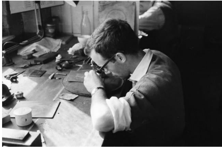
Fig 2.34. Apprentice Gerald Maudsley strengthening 61 an area of punching in a worn copper-plate, mid-1960s. CHC.
