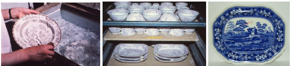
Fig. 1.14. The tissue paper is washed off leaving the colour behind. Fig. 1.15. The printed ceramics are dried-off and hardened-on in the kiln. Fig. 1.16. The ceramic is glazed and fired to produce a piece of transferware.
