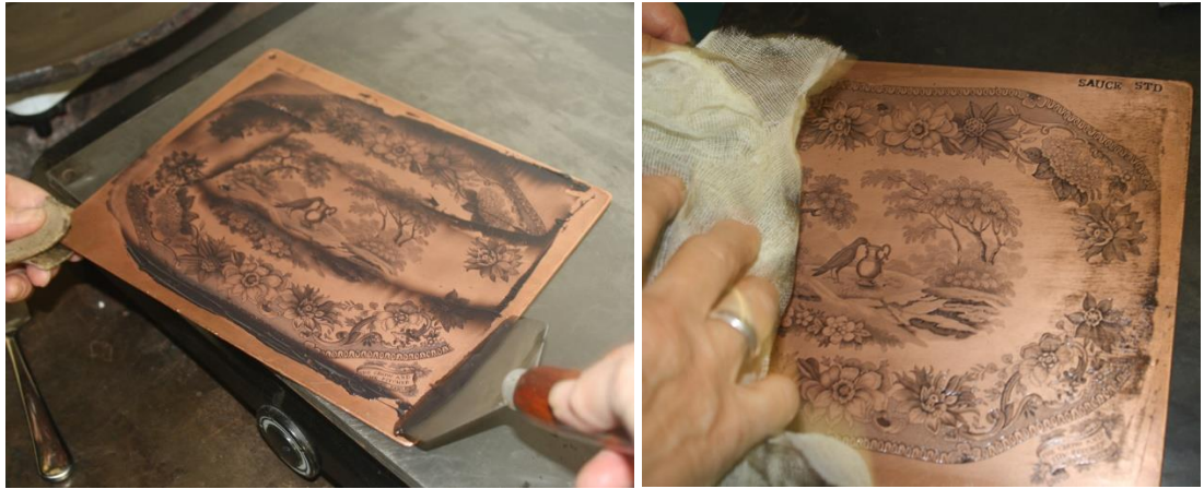
Fig. 6.57. Removal of excess colour with the scraper, and Fig. 6.58. Final removal of excess colour with cotton scrim, 2014.
