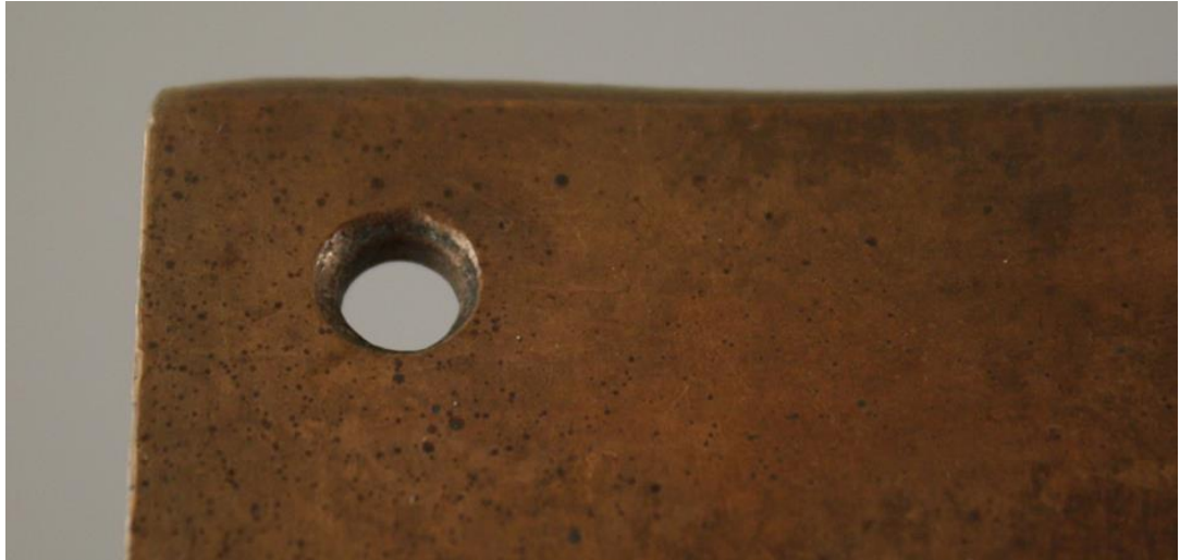
Fig. 5.89. Close-up of a drilled hole in copper-plate.
