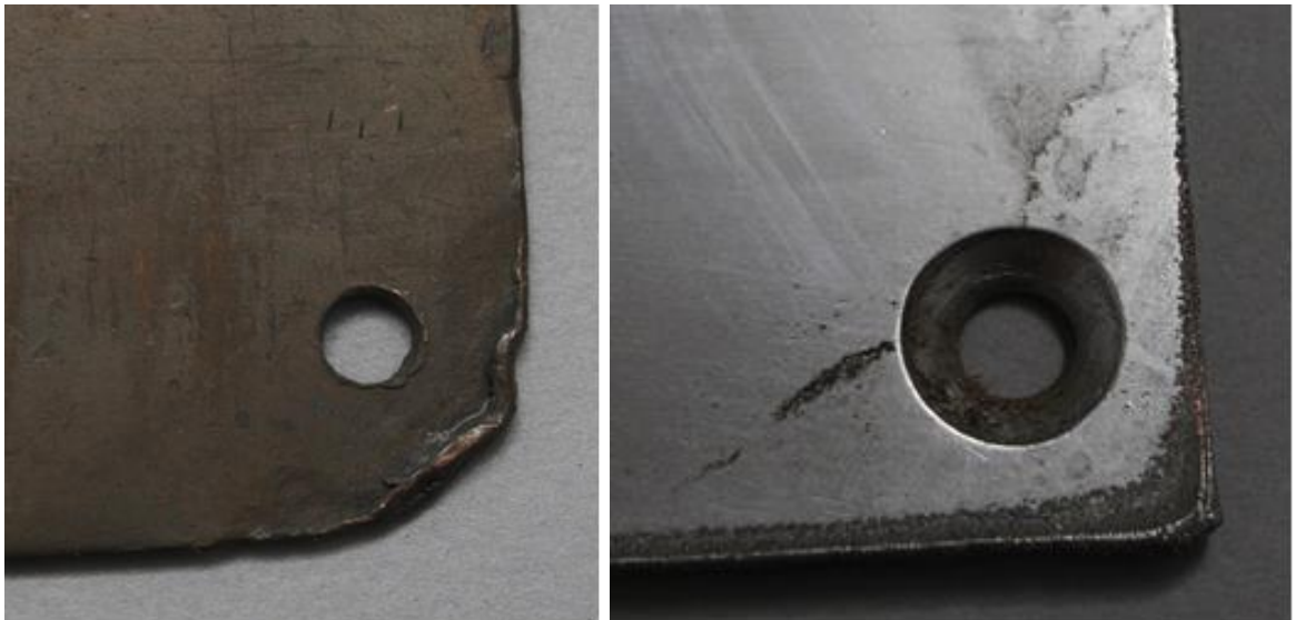
Fig. 3.108 and Fig. 3.109. Comparison of holes in copper-plates between 1820 and c.1950.
