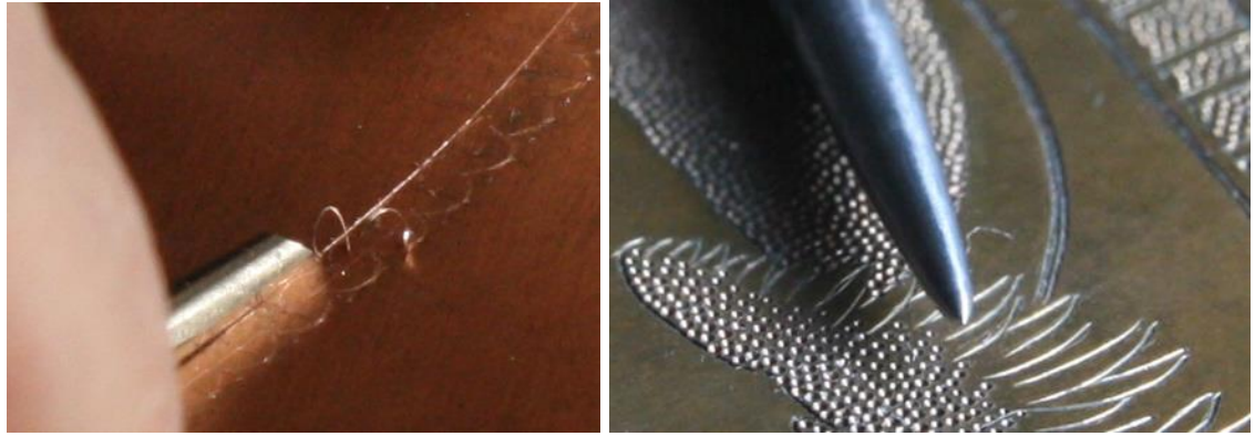
Fig. 6.132. The graver in use, and Fig. 6.133, the punch.
