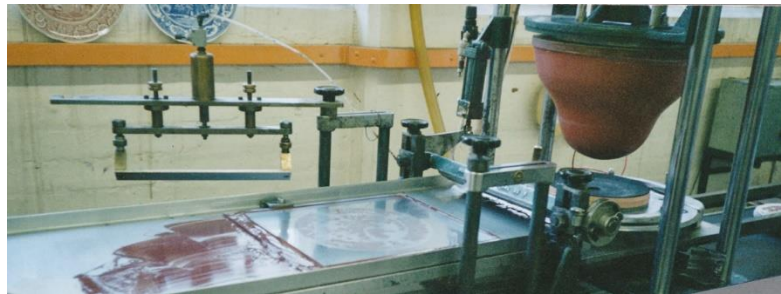
Fig. 3.93 (CHC). Close-up of the machine. From left to right: the colour tray, the chrome-plated hand-engraved copper-plate, the scraper blade, the pressing area with the silicon bomb suspended above.
