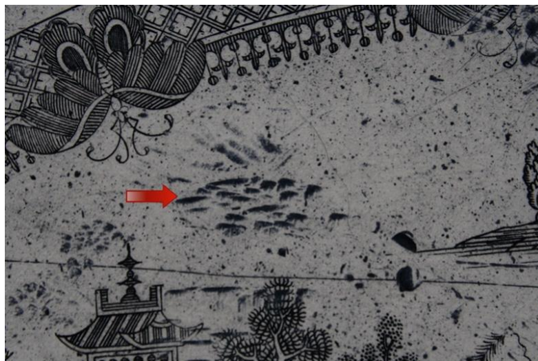
Fig. 5.33. Knocking-up transferred to a paper print.
