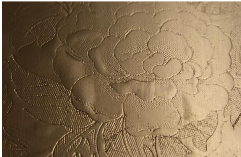
Fig. 6.86. Result of the brush forcing the foil into the engraved work.
