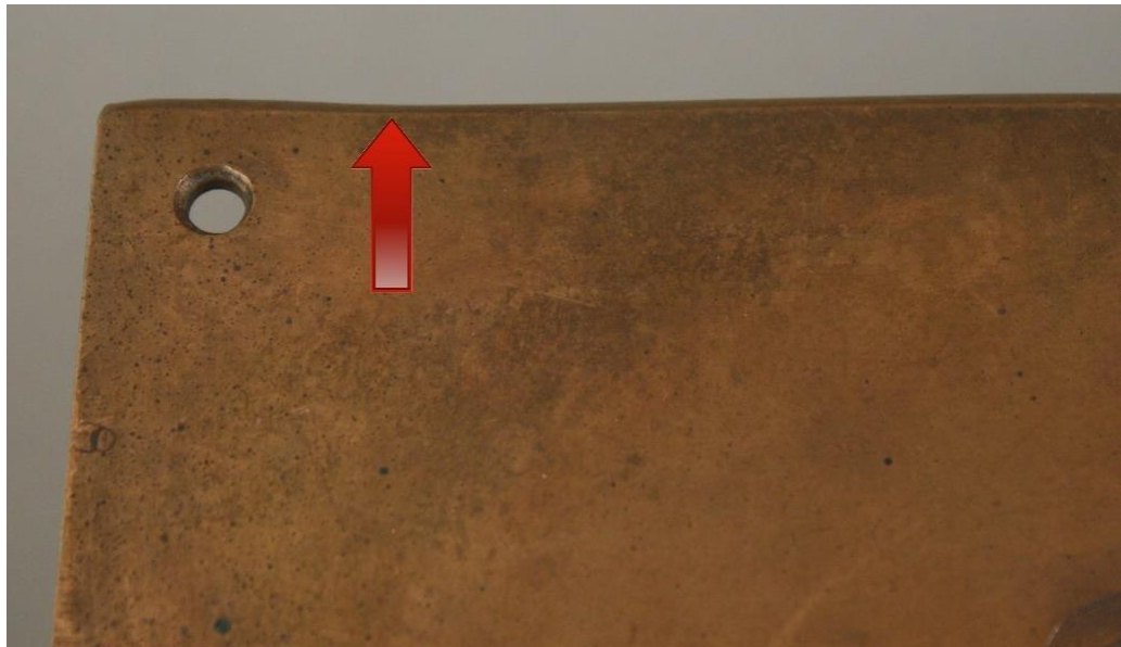
Fig. 5.88. Indicator of copper-plate that has been reduced in size.
