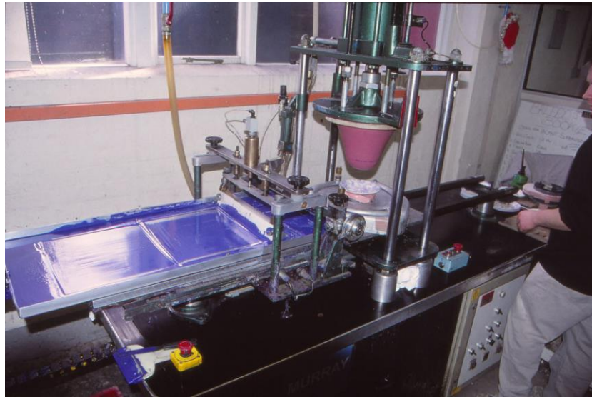
Fig. 3.97 (CHC). The printing bomb, charged with colour, moves down to the surface of the blank transferring the colour to the ware. The shape and size of the printing bomb are specific to each shape of ware.
