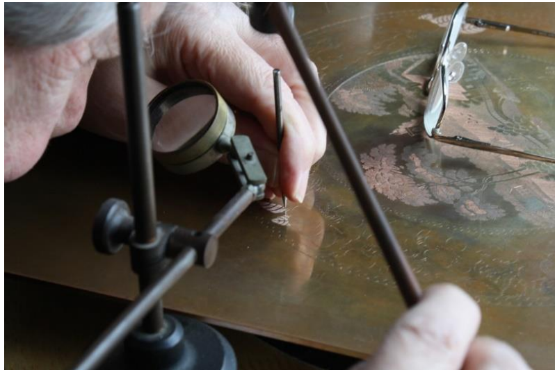
Fig. 3.25. Heath using the hammer and punch to create an area of punching. 2016.
