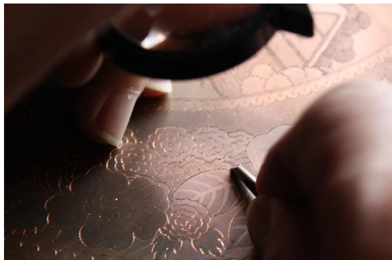
Fig. 3.22. A two-line graver being used to cut an area of cross-hatching. 2016.
