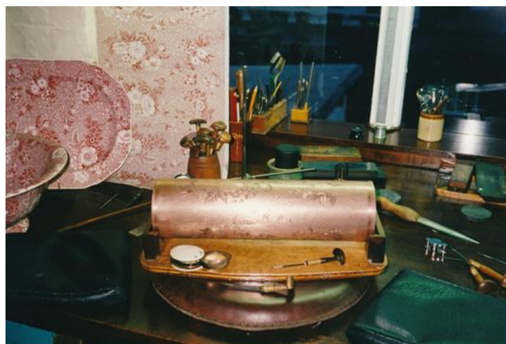
Fig. 3.82. – The finished “Primula” roller held in a wooden cradle at the workstation. CHC.
