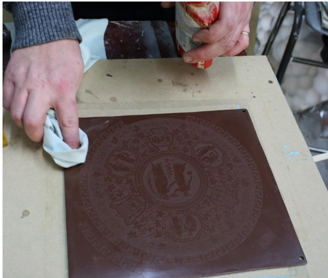
Fig. 6.112. The resin mould is polished.
