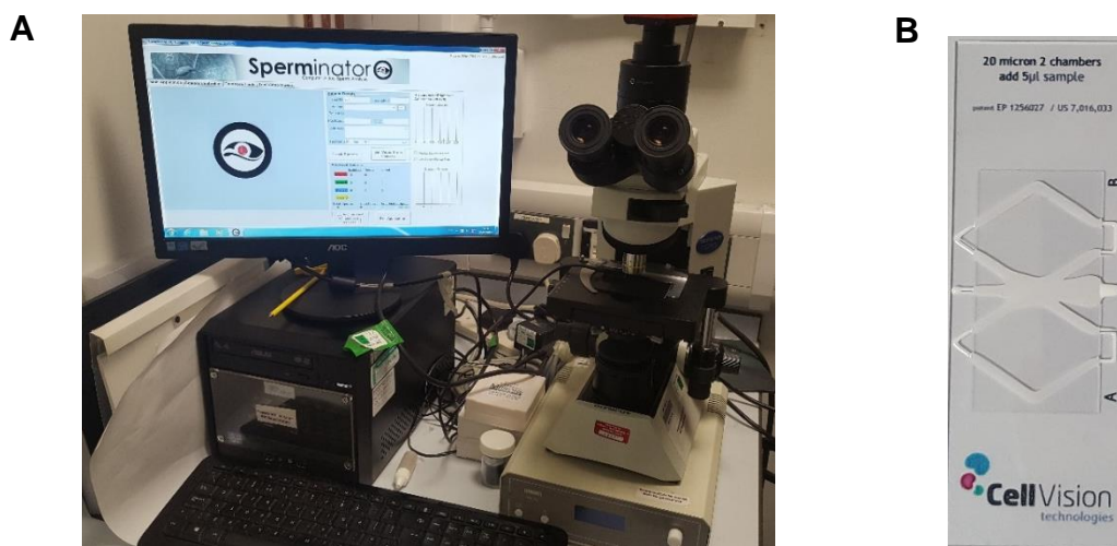
Figure 2.2: [A] Computer Assisted Sperm Analyser with Sperminator programme. [B] CASA slide.
