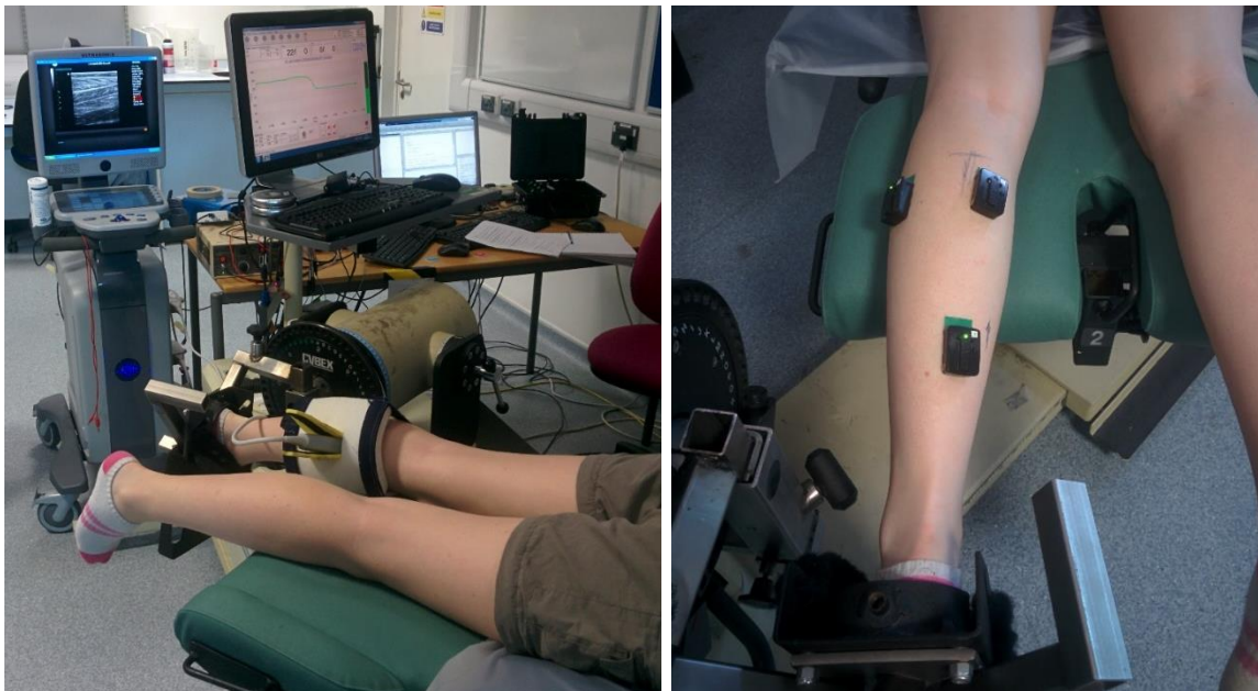
Figure 4-1. Experimental setup view including participant and US probe positioning on the dynamometer chair(left); and showing the Surface EMG electrode placement covering GM, GL and Soleus muscles of the left leg (right).
