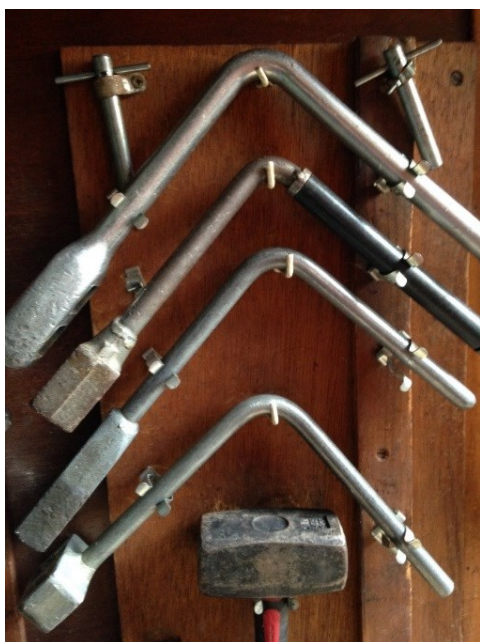
Figure 8. Anti-vandal keys (above) and windlasses on NB Olympic. Photo: Author, 2016.
