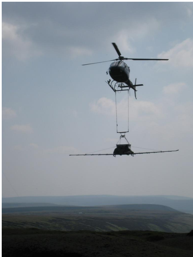
Figure 16: Helicopter spreading beads on to degraded moorlands in the Peak District
