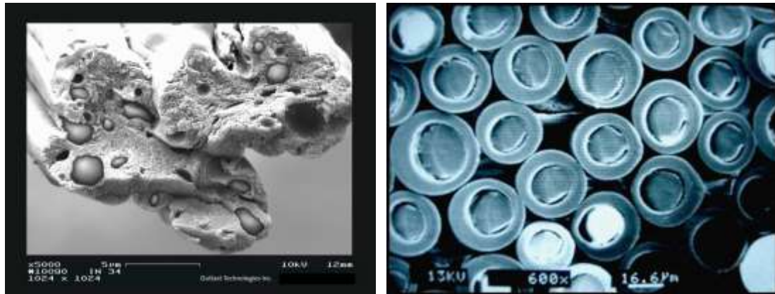
Figure 6.3: Outlast phase change material encapsulated in (i) viscose fibre and (ii) polyester fibre
