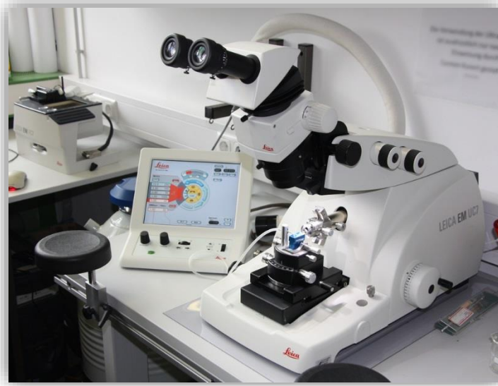
Figure A-7 Photograph of the ultramicrotome used at DiAtom to create cross sections of the SiO x coatings.
