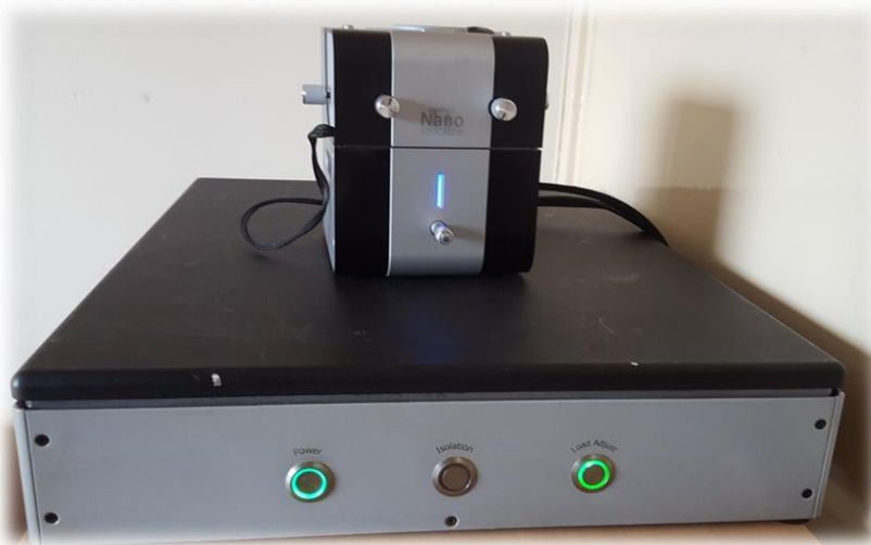
Figure A-16 Picture of the Solver Nano on a table top active vibration isolation system use for the study of prophology.
