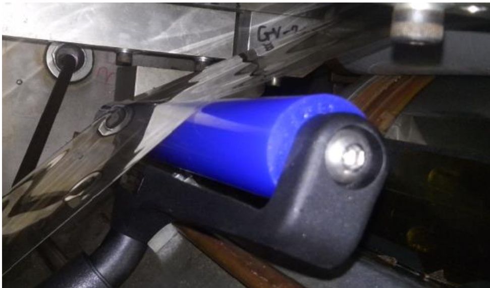
Figure 6-14 Roller located before the drum to clean the substrate before being exposed to the plasma.
