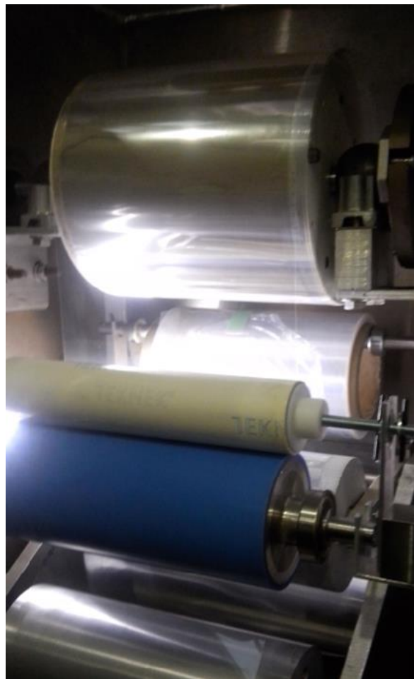
Figure 6-15 Cleaning rollers positioned in the rewind zone before the rewind roller.
