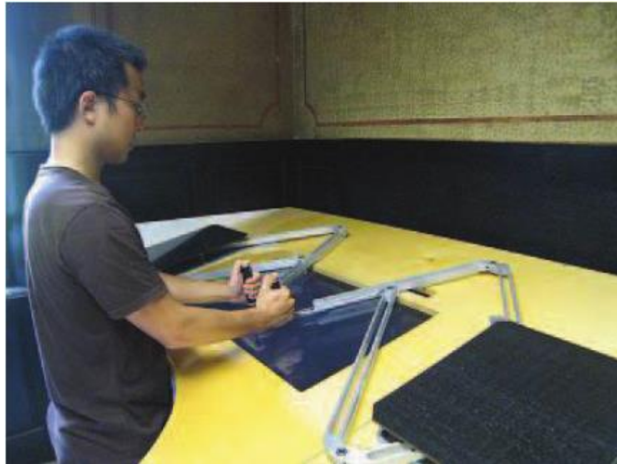
Figure 2-13: Example of a bimanual robot consisting of two single point of attachment robots. Source: (Li et al., 2009)
