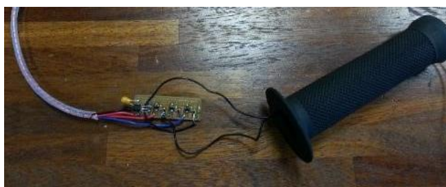
Figure A-5: The three channel capacitive sensing PCB layout
