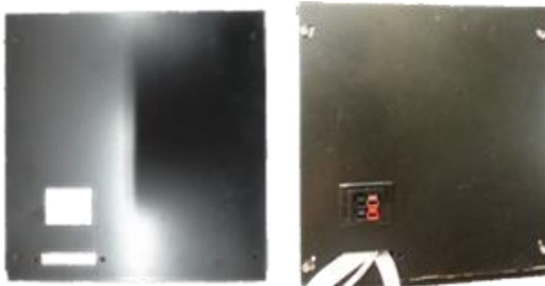
Figure A-10: Example of type of work undertaken to modify the design. The holes for the screws that attached the back plate to the main frame of the joystick were misaligned as such new holes were drilled
