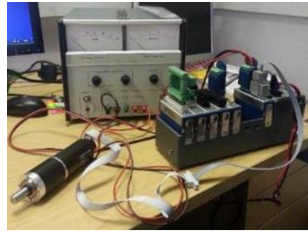
Figure A-4: Testing the interface between the motor and NI 9505
