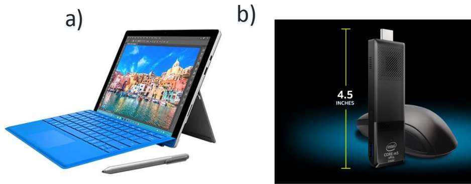
Figure 9-2: a) Examples of miniaturised computers in different form factors such as tablet computer and computer on a stick. Source a) (Microsoft Corporation, 2016) and b) (Intel Corporation, 2016)
