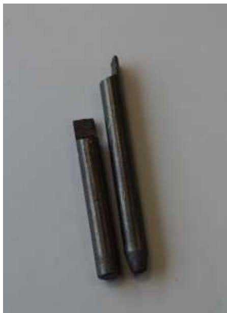
Figure 3.5.5: Pencil as electrode.
