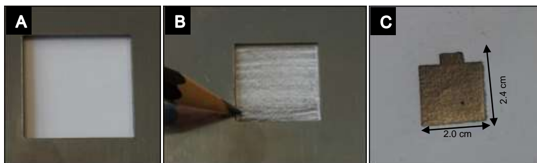
Figure 6.5.1: Bespoke metallic stencil (A) used throughout this work to create the PDEs. The PDE after one draw (B). An example of a completed PDE with connecting strip is shown in (C).
